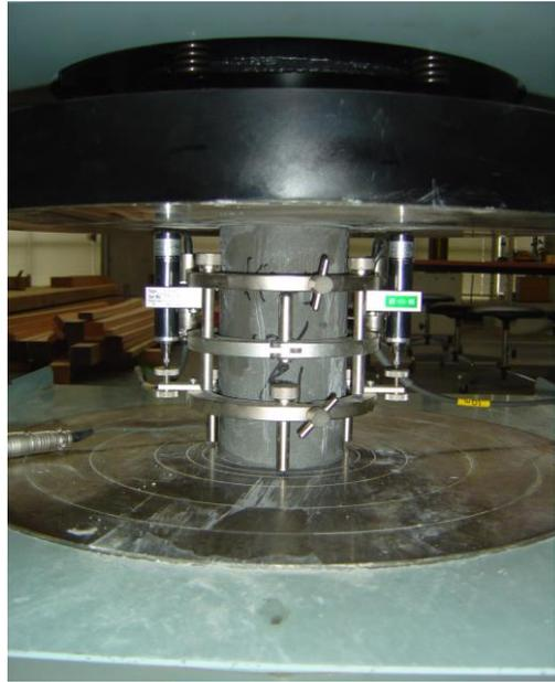
Photo 3.2 State of compressive strength test
