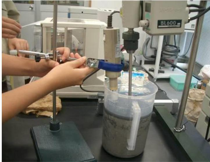
Figure 4.2. Microbubble generator.
