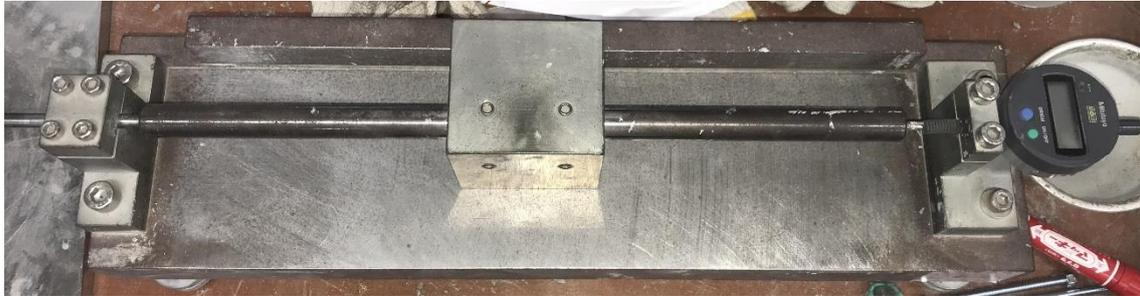
Photo 3.5 Drying shrinkage test equipment
