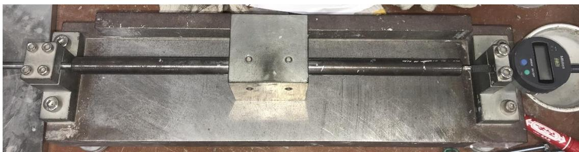
Photo 7.2 Drying shrinkage test equipment
