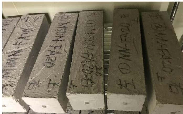
Photo 3.3 State of drying specimen in curing room
