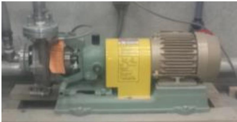
Figure 4.6. The medium unburned carbon removal device.
