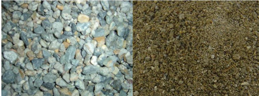
Photo 2.1. Recycled coarse aggregate and recycled fine aggregate [2]
