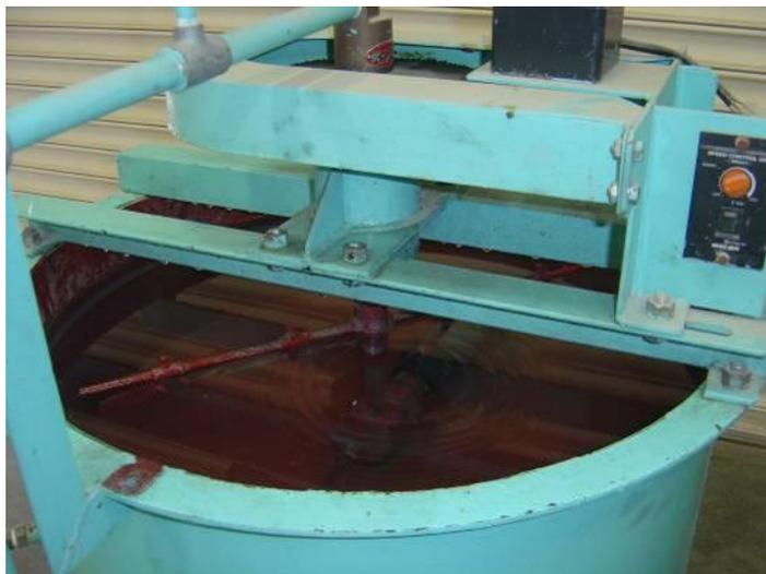
Figure 4.1. The flotation device of the air diffuser.
