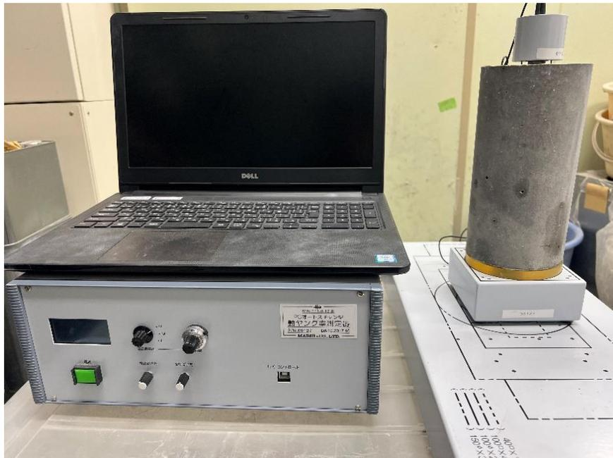
Photo 3.6 Dynamic elastic modulus test machine.
