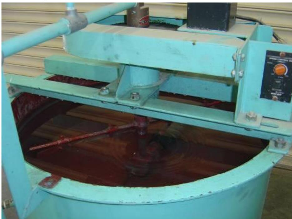
Figure 3.1. The flotation device of the air diffuser.
