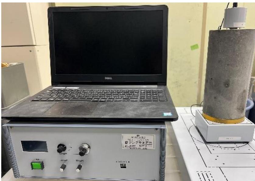
Picture 6.2. Test device for  $E_d$ .
