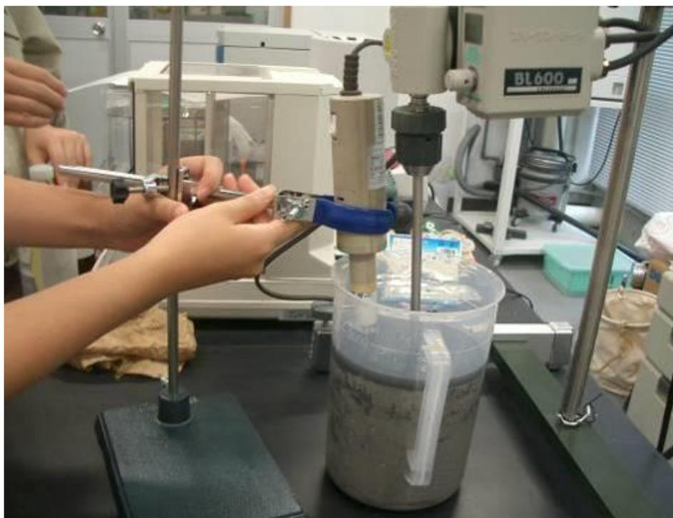
Figure 3.2. Microbubble generator.
