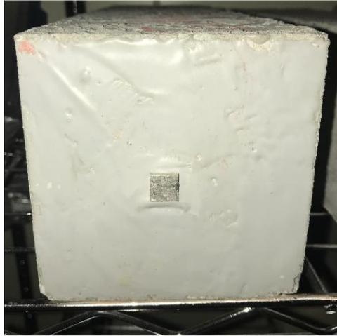
Photo 3.4 The gauge plug in the specimen
