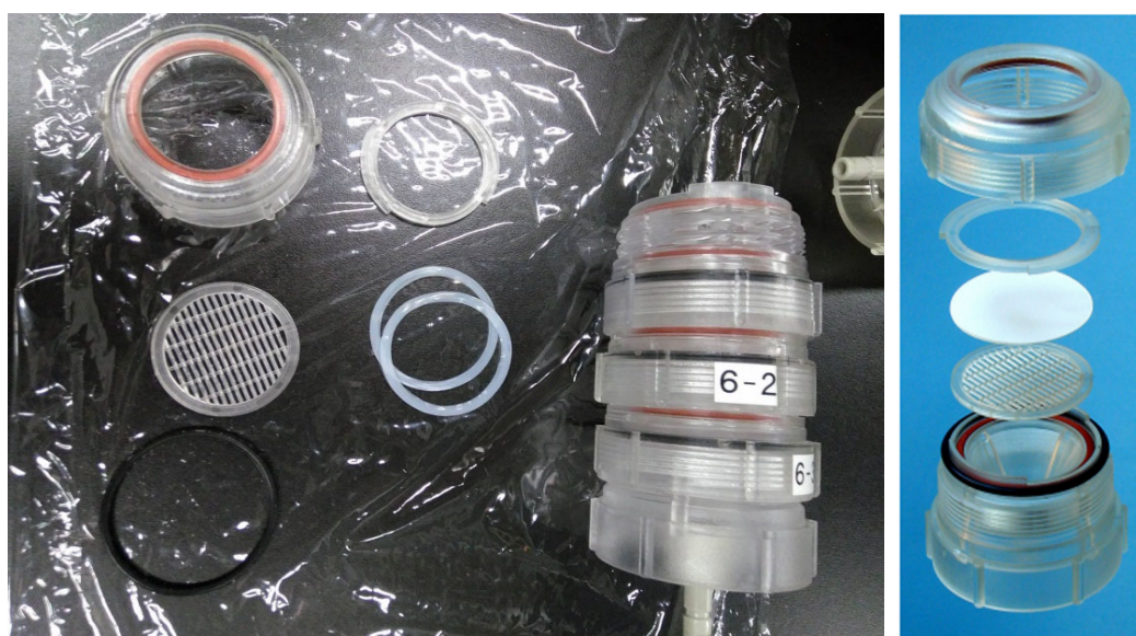
Fig. 1-5 A NILU four-stage filter holder and assembly in one stage ( www.innovation.nilu.no )
