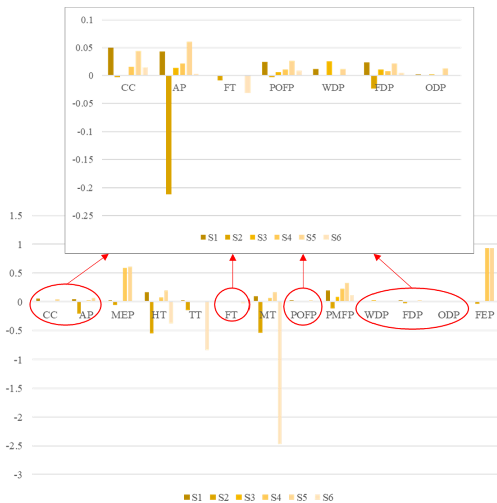
Fig. 3.4 Net environmental impact of each scenario for sewage sludge recycling system (Note: CC: kg CO 2 eq, TA: kg SO 2 eq, MEP: kg N eq, FEP: kg P eq, HT, kg 1,4-DB eq, TT: kg 1,4-DB eq, FT: kg 1,4-DB eq, MT: kg 1,4-DB eq, POFP: kg NMVOC eq, PMFP: kg PM10 eq, WDP: m 3 , FDP: kg oil eq, ODP: kg CFC-11 eq)
