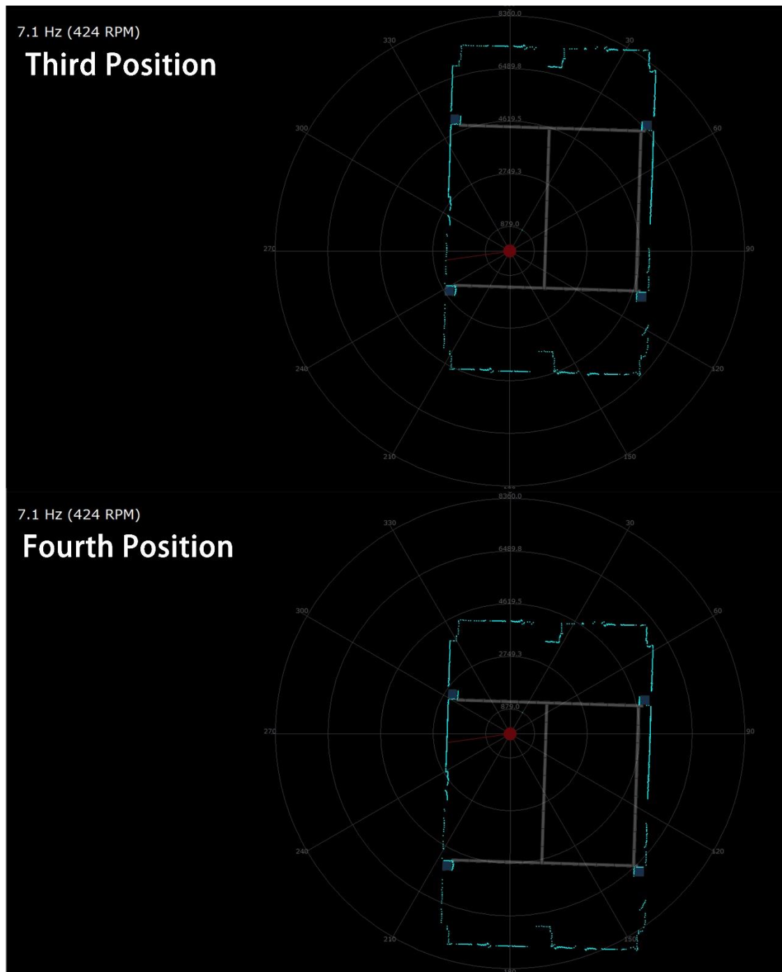
Fig. 5-32 (b) Scanning and alignment of the robot's four positioning points.
