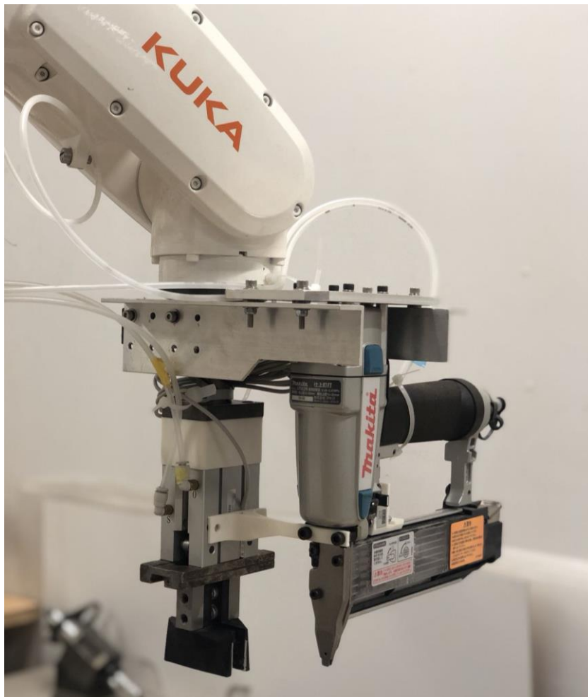
Fig. 3-14 The end-effector of KUKA robot in the case study.
