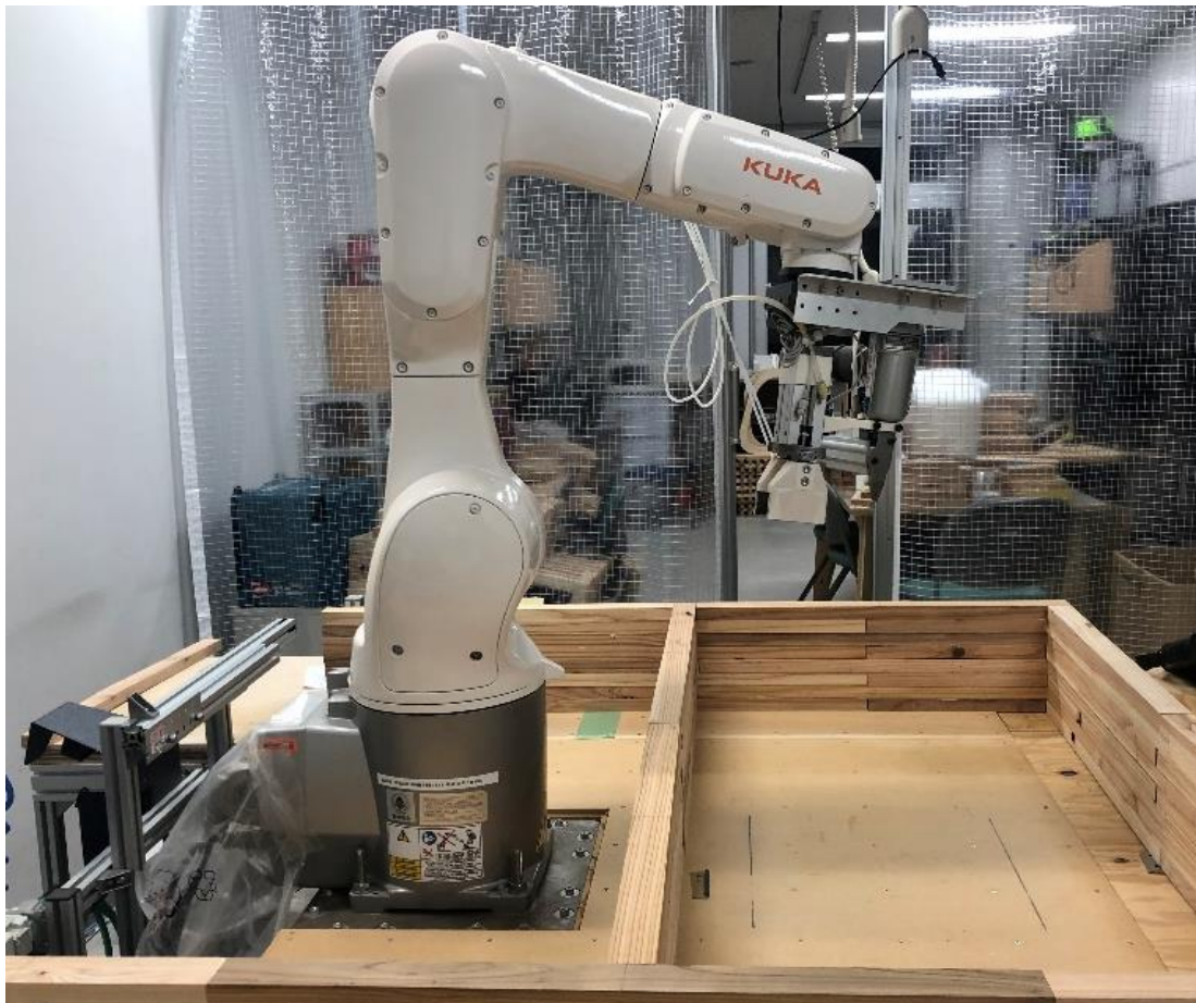
Fig. 4-3 The construction robotic set-up is customized for the fabrication of timber buildings.
