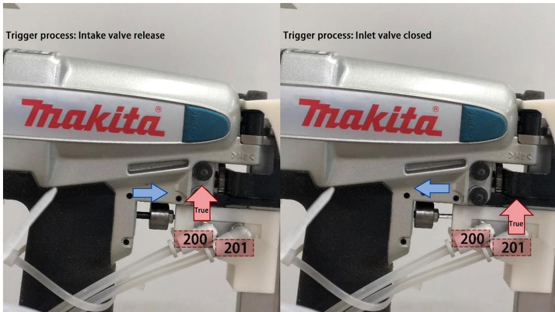
Fig. 4-32 Implementation process of program operated air nail gun.
