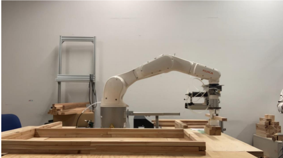
Fig. 4-48 Live photos of robot nailing action.
