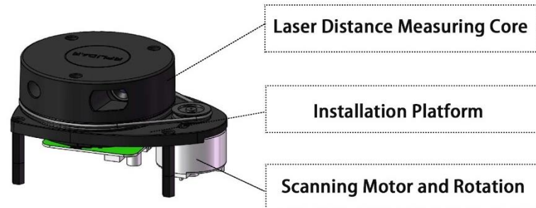
Fig. 5-28 RPLIDAR A1 system configuration diagram.
