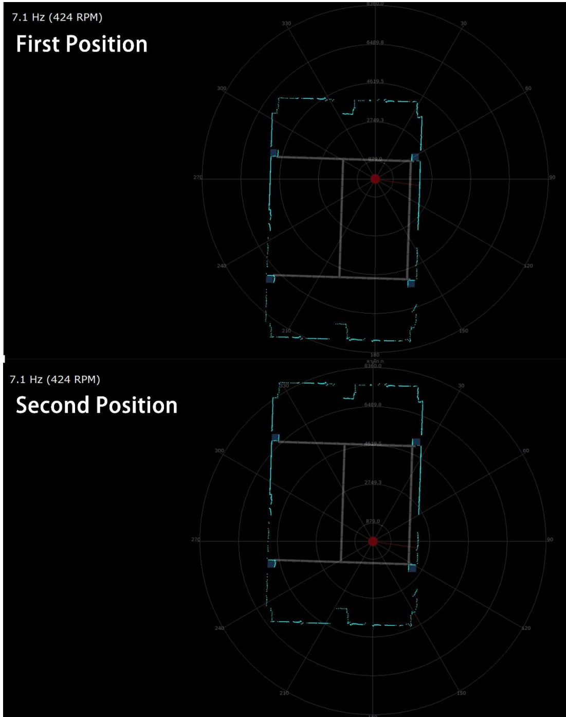
Fig. 5-32 (a) Scanning and alignment of the robot's four positioning points.
