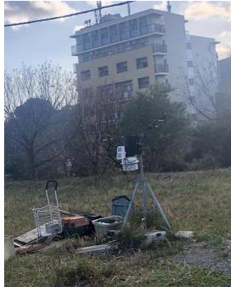
**Figure 3.1.4 The picture of Davis Vantage Pro2 and Installation location**
