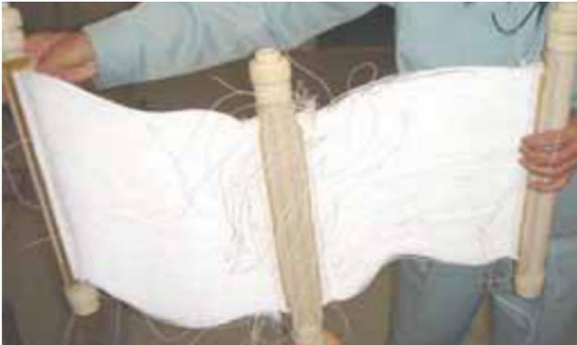
Fig 2-18 The hollow fiber membrane (part) in the MBR of the HRG
