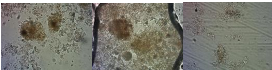
Figure 3-15. Morphological observation of microorganisms in activated sludge when VFL treats landfill leachate (400 times, in order: anaerobic stage, anoxic stage, aerobic stage).
