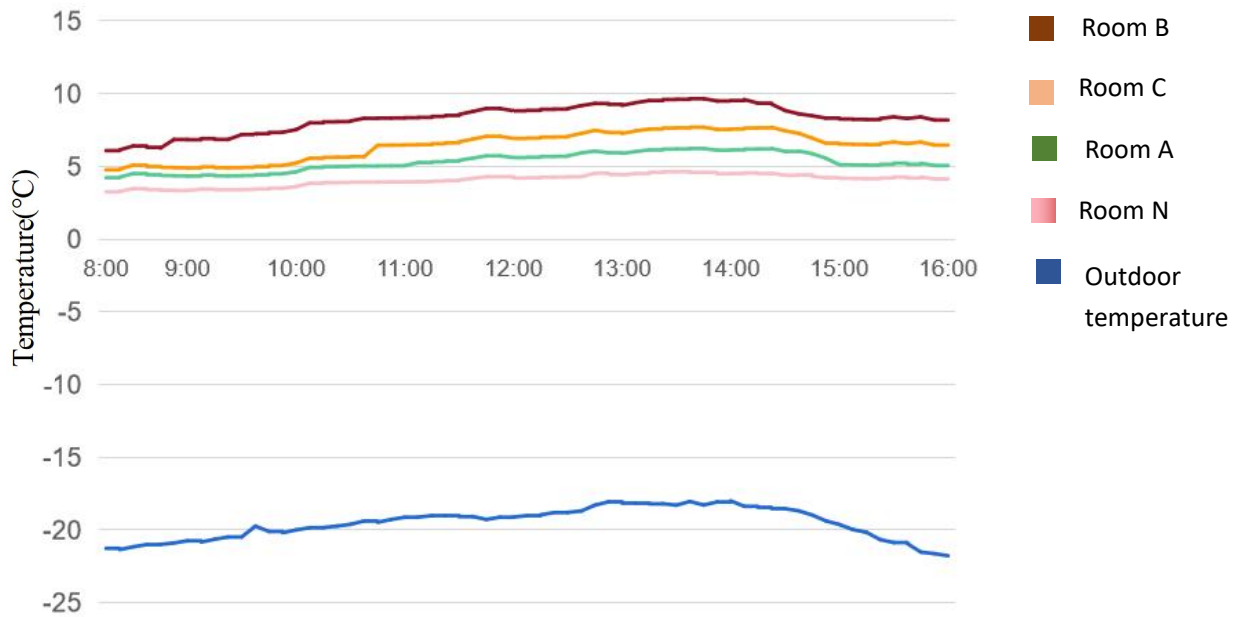
Fig 5-6 Inter Room temperature in different circulation modes with DC fans off
