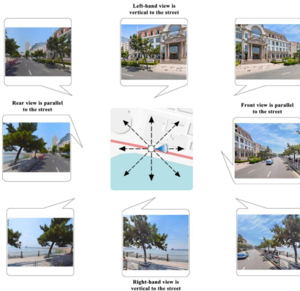
**Fig 3-1 Street View Image Acquisition Example Diagram**
