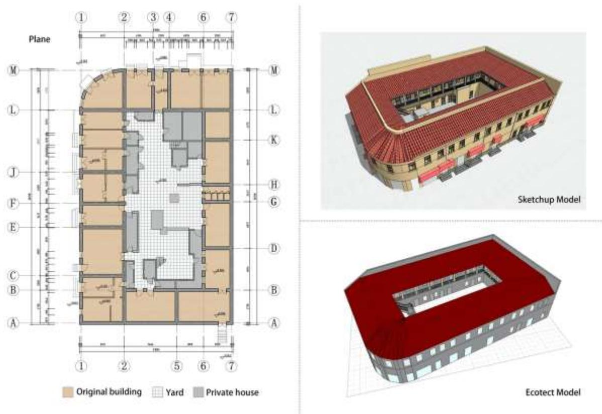
Figure 6-1. SketchUp model, simulation model, and plane of the Liyuan house in Qingdao
