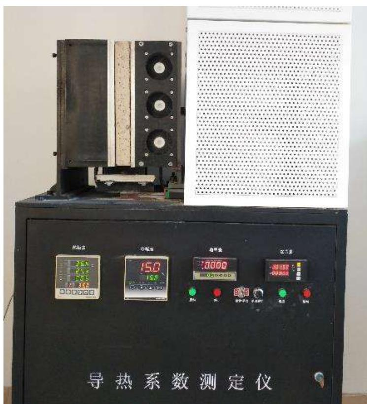
Figure 3-3. The appearance thermal conductivity tester
