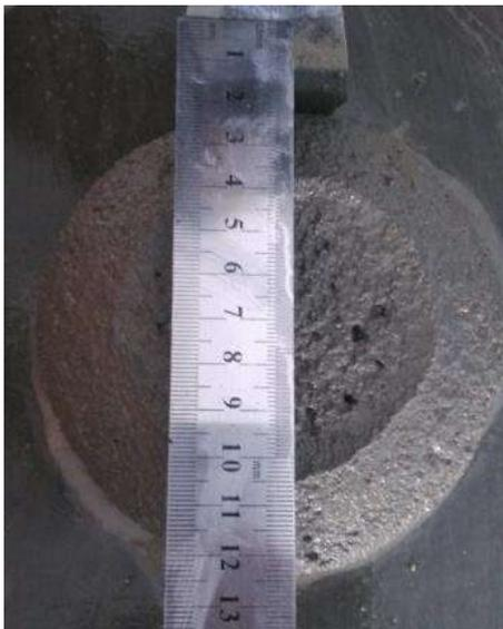
(b) Measurement of fluidity of reclaimed mortar
