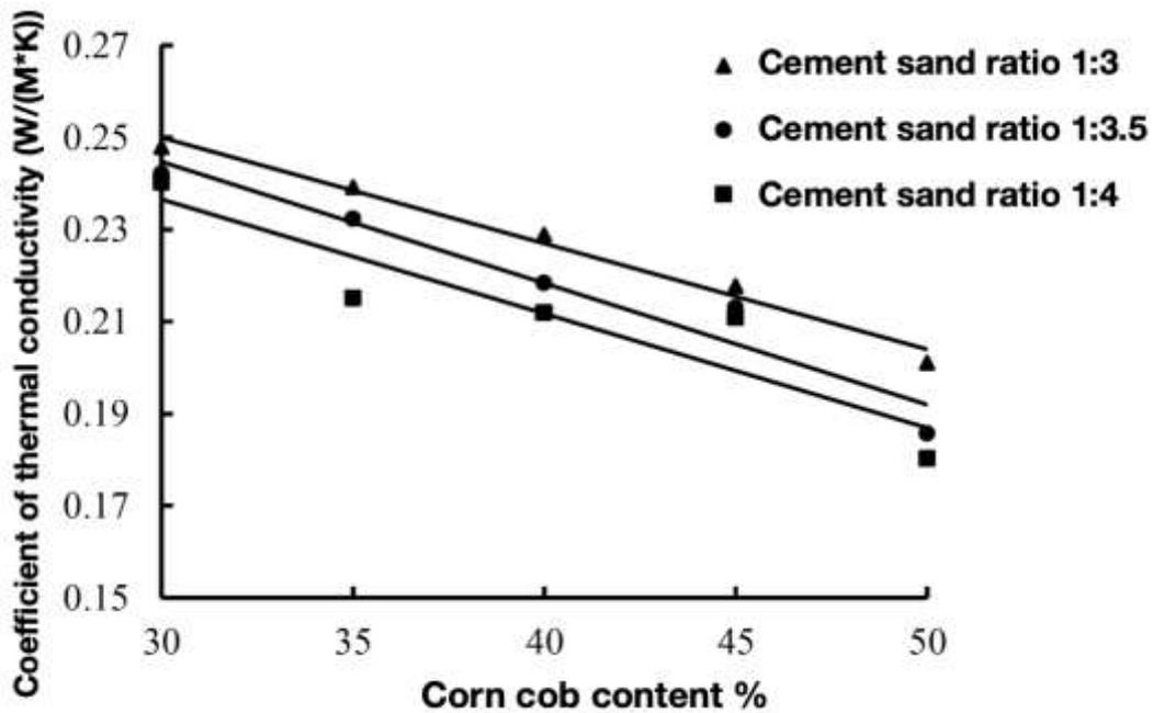
Figure 5-10. The thermal conductivity curve to the corncob volume content
