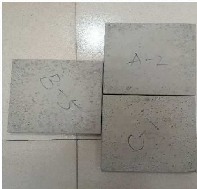
Figure 3-2. The concrete heat conduction board after drying
