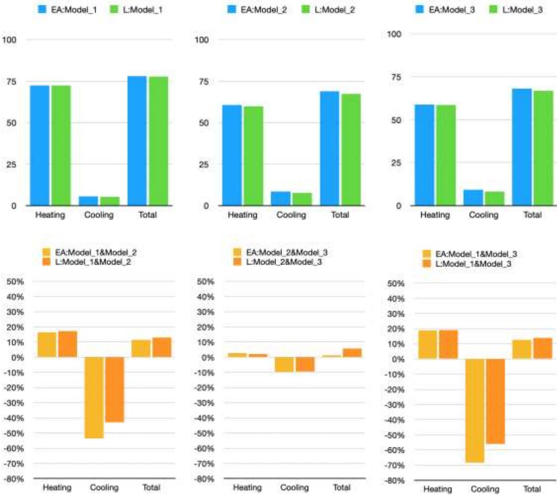
Figure 6-18. Comparison of data from Ecotect analysis and ladybug +honeybee software
