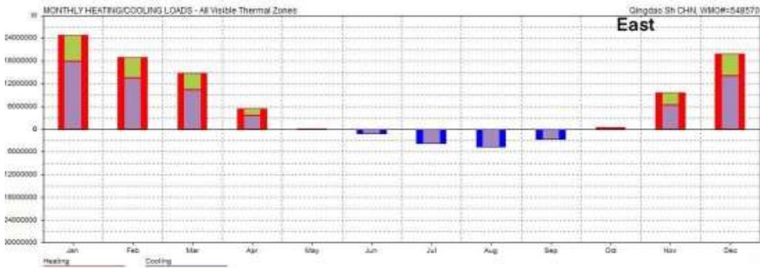
Figure 6-26. The monthly heating and cooling when change EAST facade
