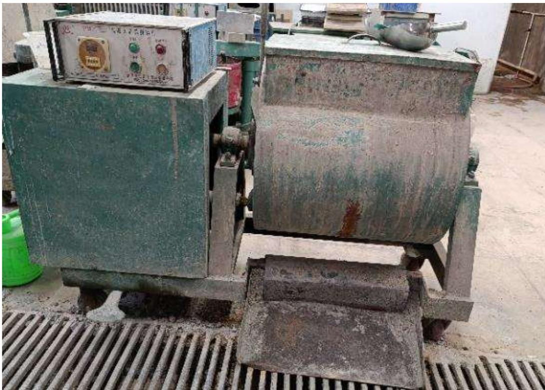
Figure 5-6. The concrete horizontal mixer
