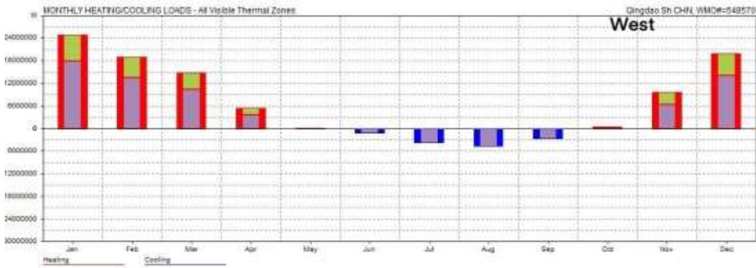
Figure 6-27. The monthly heating and cooling when changes WEST facade
