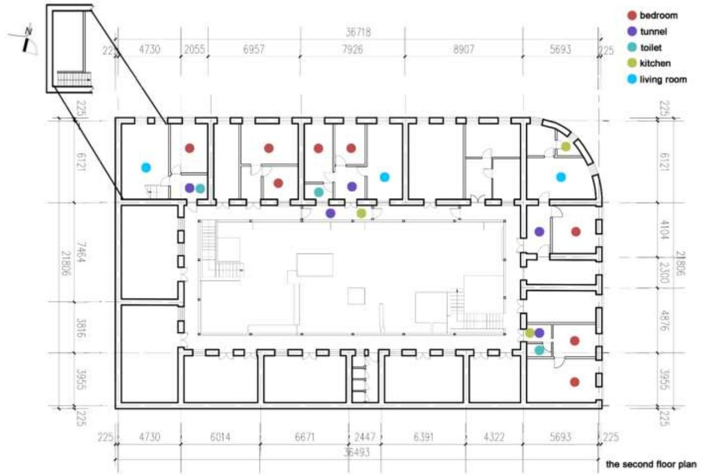
Figure 4-11. The detailed layout of the 2nd floor in Case A
