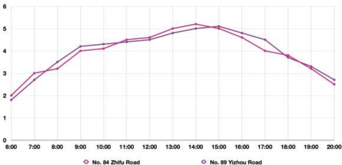
Figure 4-20. The comparison of indoor temperature change curves between two Liyuan courtyards
