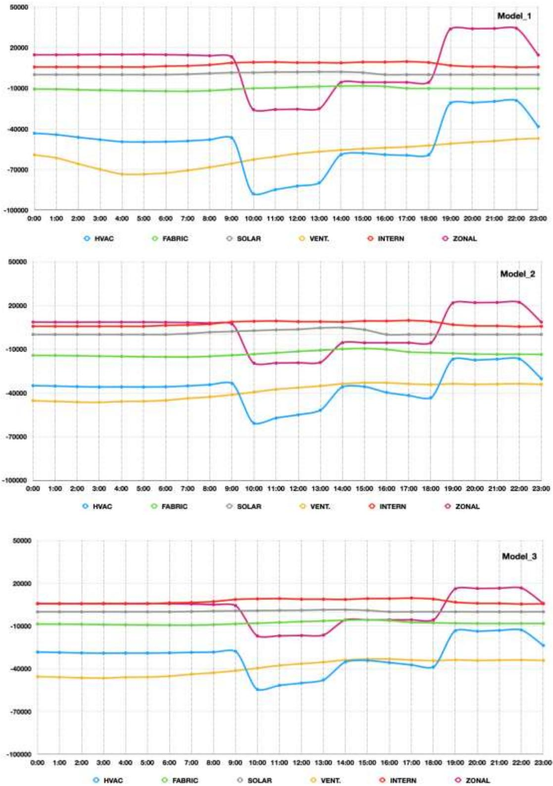
Figure 6-7. The hourly heat gains or losses result sheets of the three models
