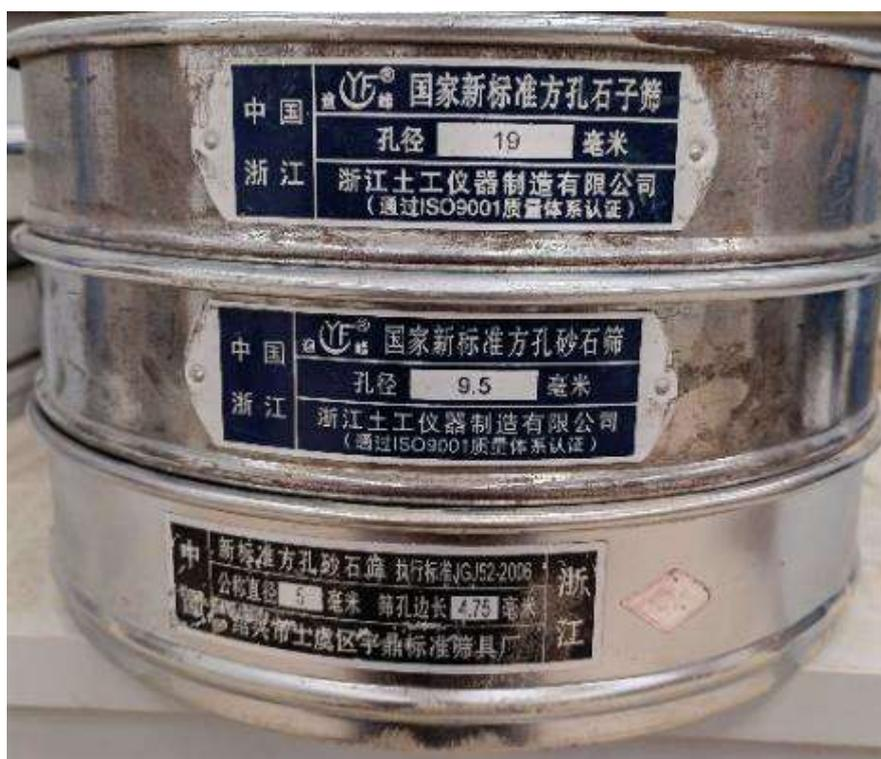
Figure 5-3. The standard square hole sieve
