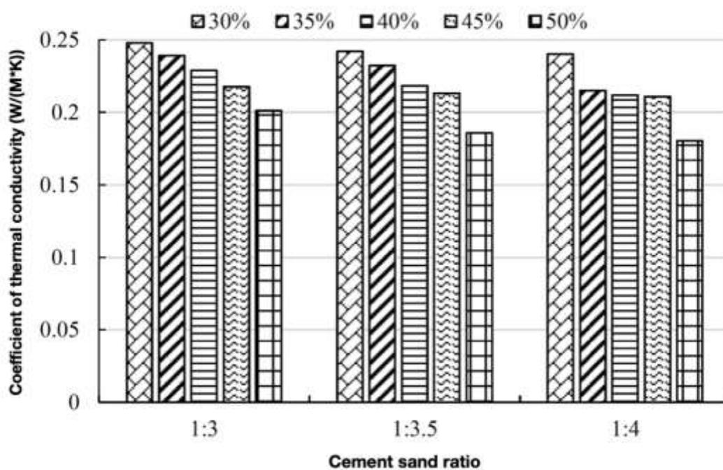
Figure 5-11. The relationship between the cement sand ratio and the thermal conductivity
