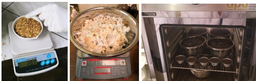
Figure 27. Materials Preparations: Rice Husk, Shredded Disposable Diapers and Aggregates
