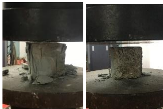
Figure 35. Compressive strength of cement based composite mortar
