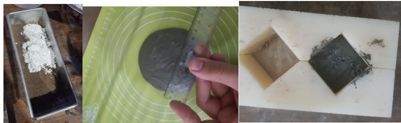
Figure 34. Measurement of slurry diameter to determine the workability of mortar.
