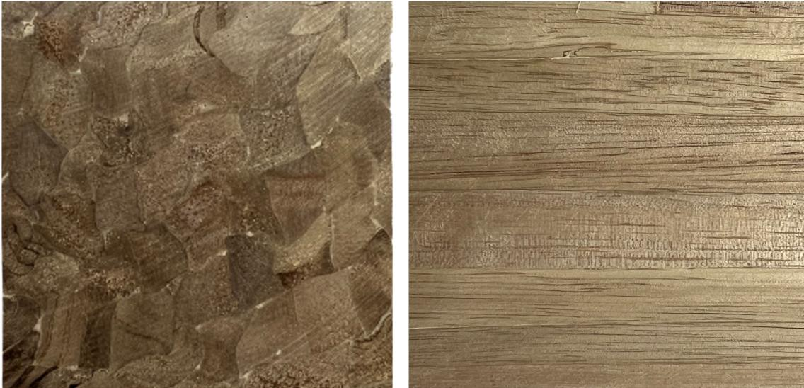
Figure 7. 13 Treated albasia wood (Left: Cross section); (Right: Fiber direction).
