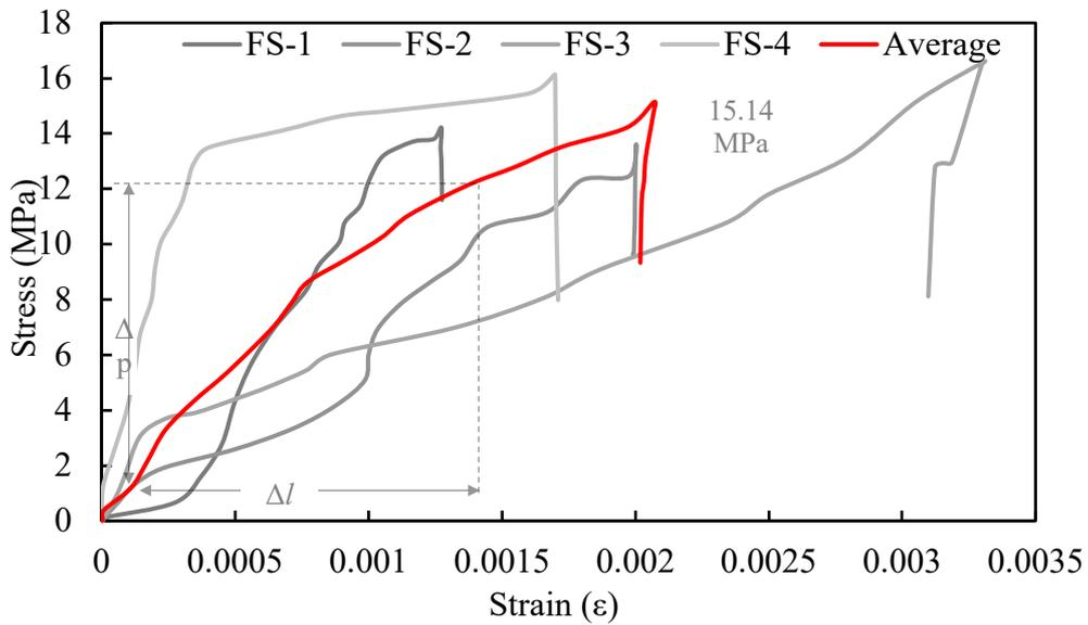
Figure 6. 39 Relationship between stress (MPa) and strain ( $\epsilon$ ) of of treated wood (albasia Voronoi composite) in tangential direction compressive strength.
