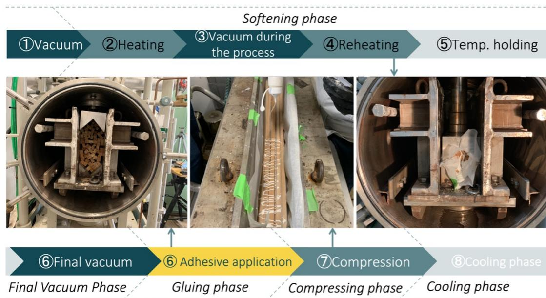
Figure 6. 9 Consolidation illustration of Albasia Voronoi composite wood.
