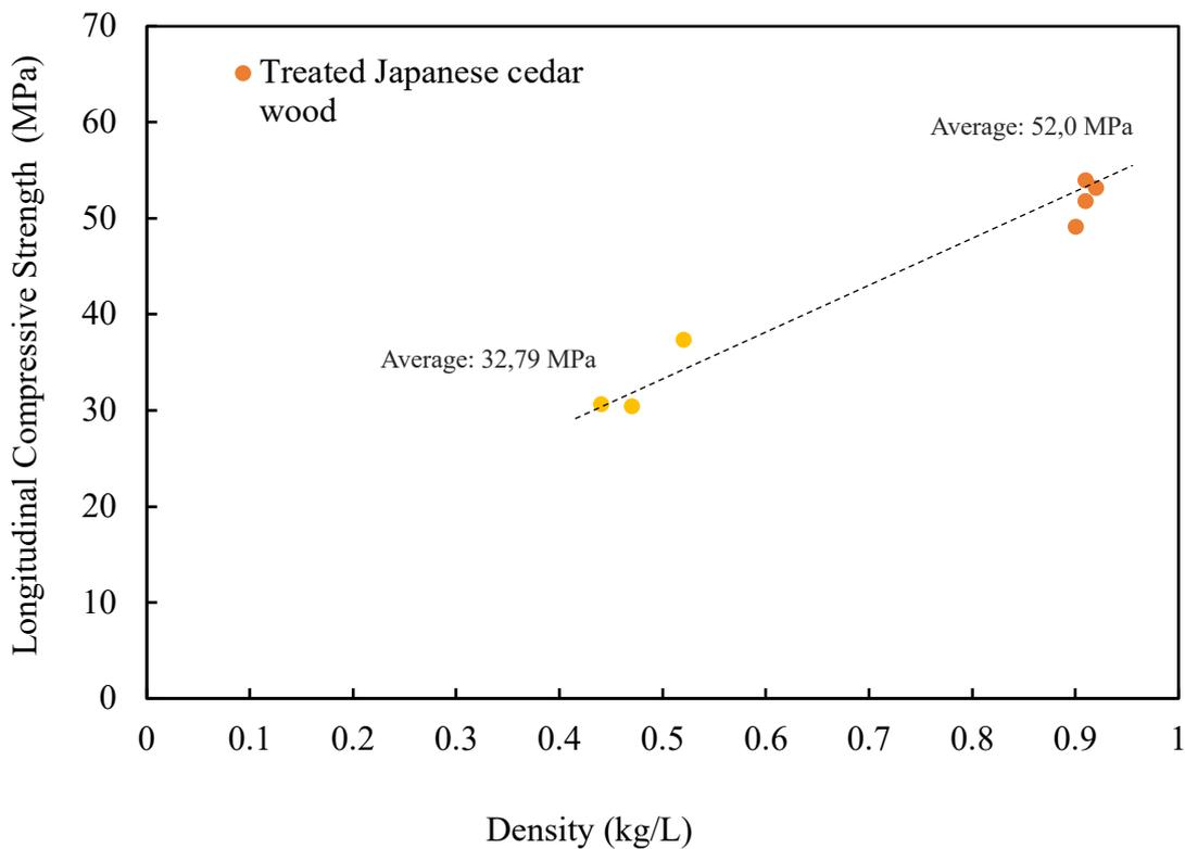
Figure 7. 18 Correlation between specific gravity and longitudinal compressive strength of treated and untreated Japanese cedar.
