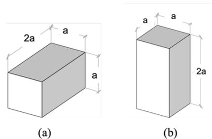
Figure 3. 20 The dimension of a wood sample for the compressive strength
