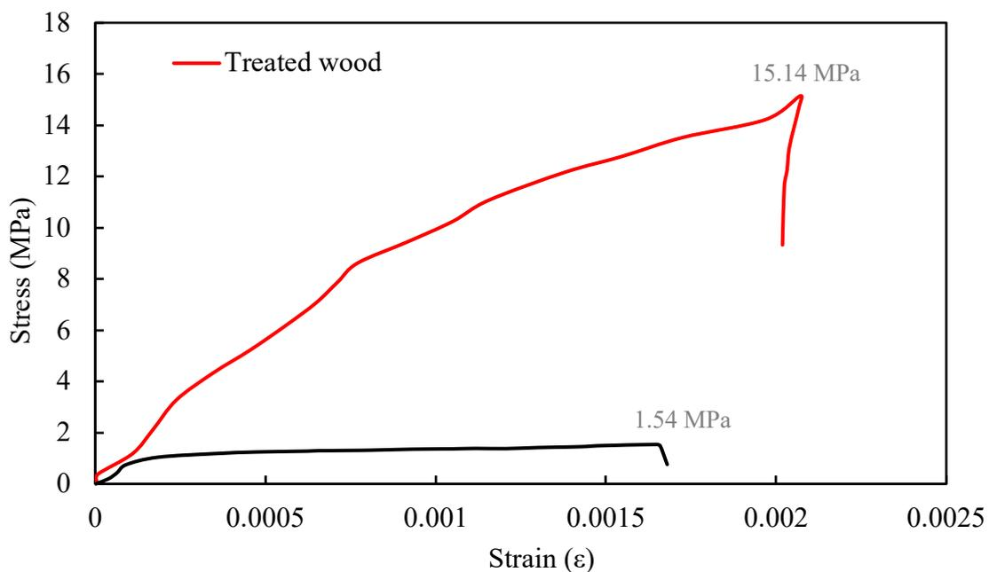
Figure 6. 41 Comparative relationship between stress (MPa) and strain ( $\epsilon$ ) of treated and control wood in tangential direction compressive strength test.
