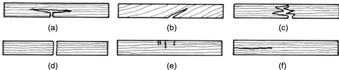
Figure 6. 48 Failure types of clear wood in bending with span parallel to grain: (a) simple tension, (b) cross-grain tension, (c) splintering tension, (d) brush tension, (e) compression, (f) horizontal shear.
