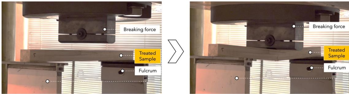
Figure 6. 47 Longitudinal bending strength test on treated wood.
