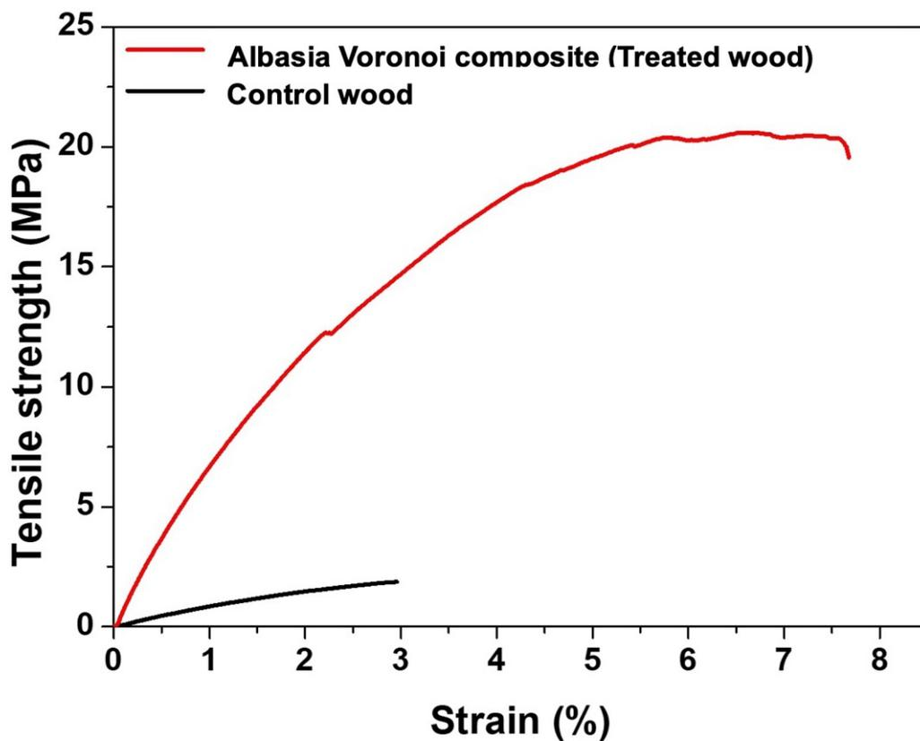
Figure 6. 54 Relationship curves between tensile stress and strain of control and treated wood (albasia Voronoi composite).
