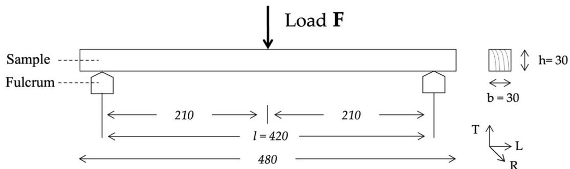
Figure 7. 11 Schematic Illustration for three-point bending tests. Dimensions are presented in mm.
