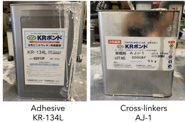
Figure 6. 6 Adhesive and Isocyanate (Cross linker) used in the experiment.
