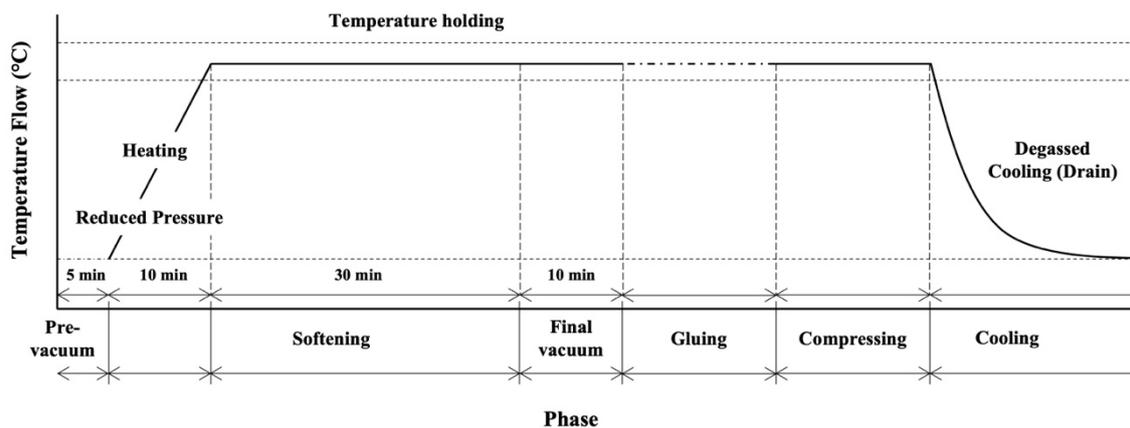
Figure 6. 8 Consolidation process of Albasia Voronoi composite wood.
