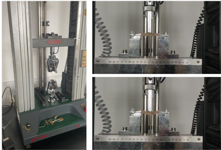
Figure 3. 23 Universal material testing machine CMT6104 for bending strength test.
