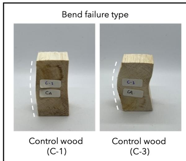
Figure 6. 43 Bend failure type of wood in compressive strength test tangential direction on control wood
