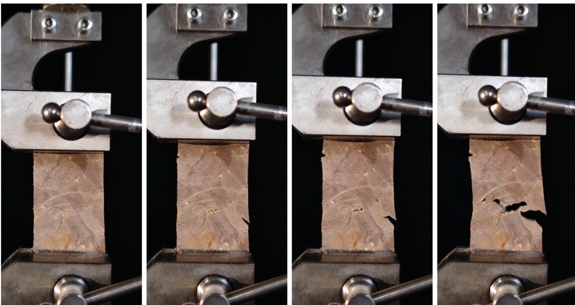
Figure 6. 57 Tensile test on treated wood.
