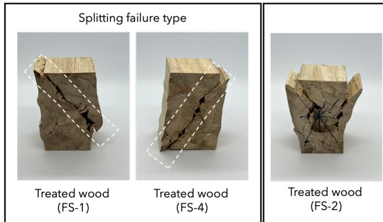
Figure 6. 42 Splitting failure type of wood in compressive strength test tangential direction on treated wood (albasia Voronoi composite)
