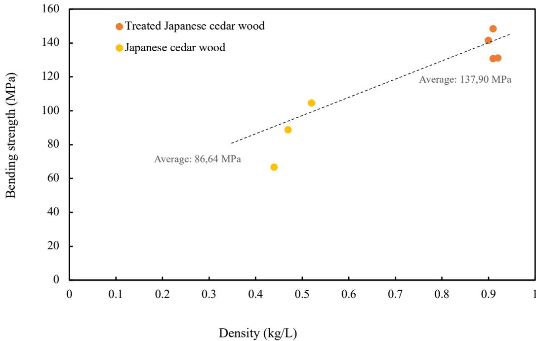
Figure 7. 25 Correlation between specific gravity and bending strength of treated and untreated Japanese cedar wood.
