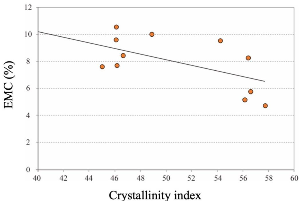
Figure 2. 7 Correlation between crystallinity index and EMC
