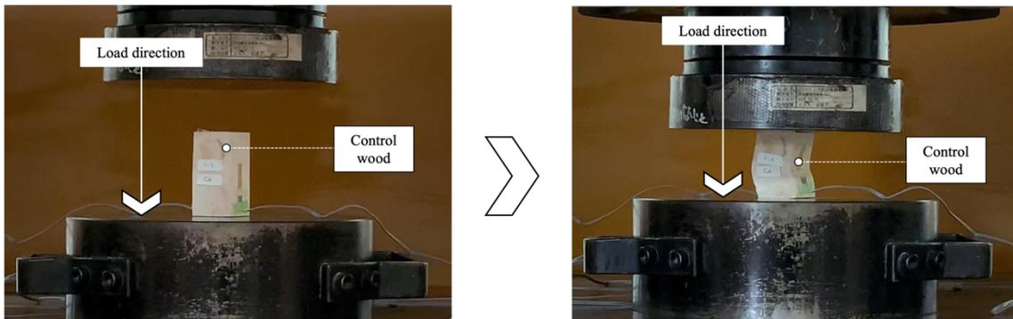
Figure 6. 37 Tangential compressive strength test on the control wood
