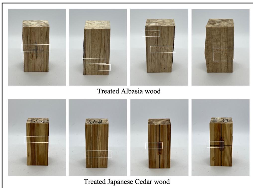
Figure 7. 16 Representative photographs of typical failure patterns of treated albasia and Japanese cedar wood longitudinal compression test.
