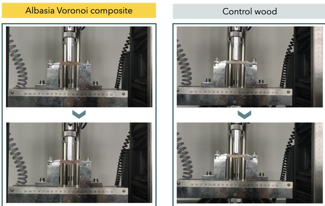
Figure 6. 51 Tangential bending strength on control and treated wood.
