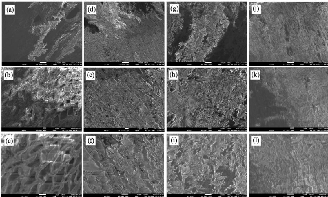
Figure 5. 10 SEM micrographs: control (a) 100 "μm" , (b) 500 "μm" , (c) 1000 "μm" ; 100 °C (d) 100 "μm" , (e) 500 "μm" , (f) 1000 "μm" ; 120 °C (g) 100 "μm" , (h) 500 "μm" , (i) 1000 "μm" ; 140 °C (j) 100 "μm" , (k) 500 "μm" , (l) 1000 "μm."
