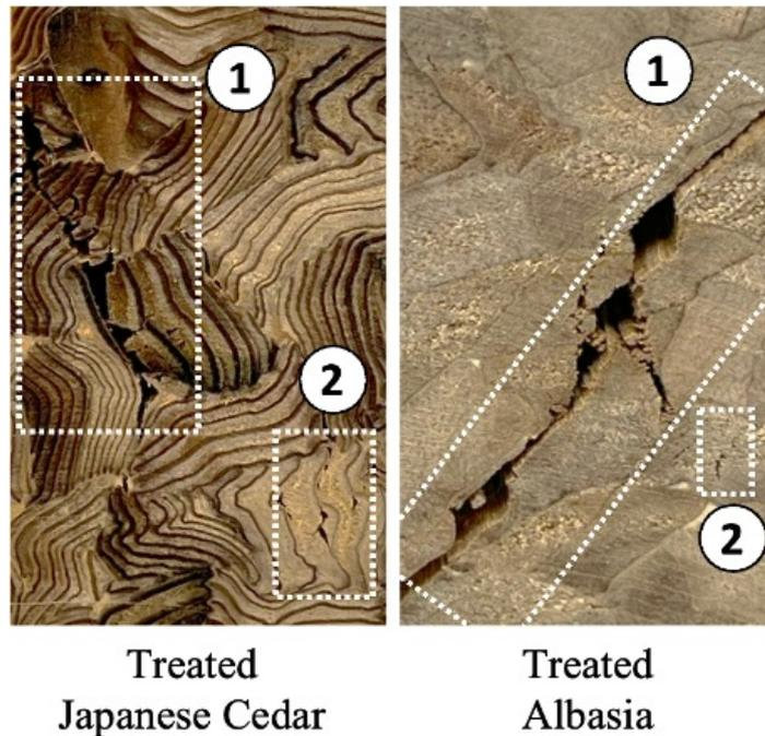
Figure 7. 23 A close-up view of cracks and fractures in the specimen after compressive strength test.
