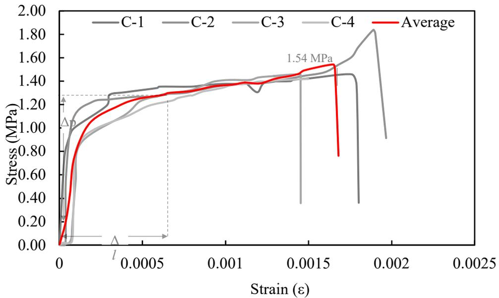
Figure 6. 40 Relationship between stress (MPa) and strain ( $\epsilon$ ) of control wood in tangential direction compressive strength.
