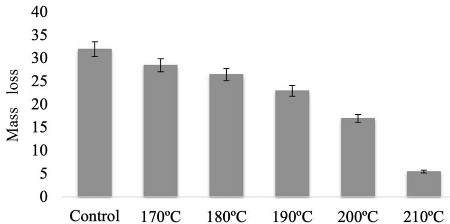
Figure 2. 8 Correlation of mass loss in modified and modified poplar wood caused by soft-rot fungi
