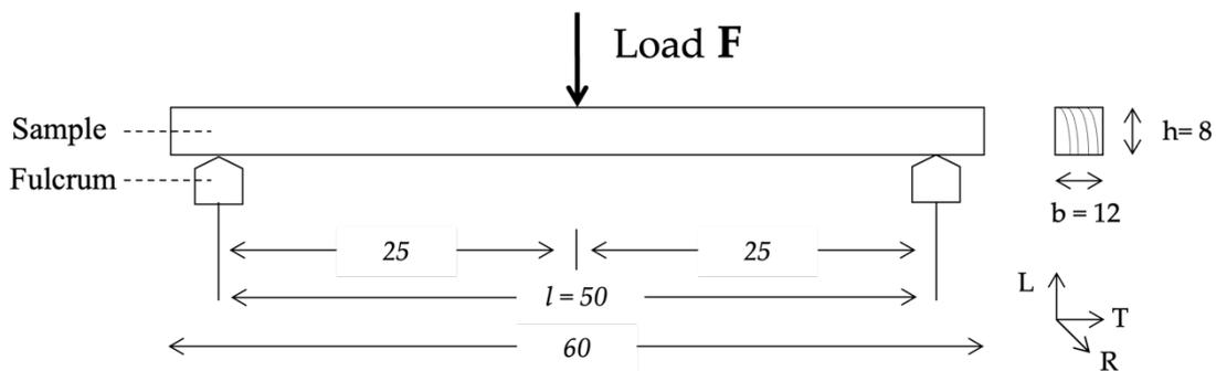
Figure 6.16 Schematic Illustration for three-point tangential bending tests.
