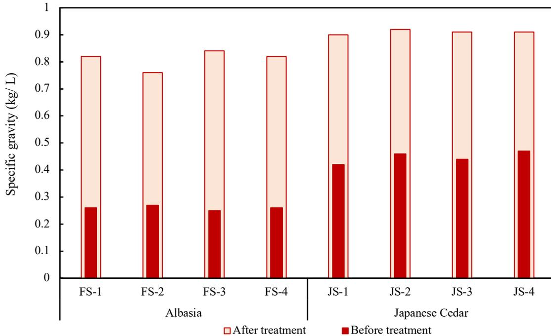
Figure 7. 15 Comparison of the increase in density of albasia and Japanese cedar wood before and after treatment.
