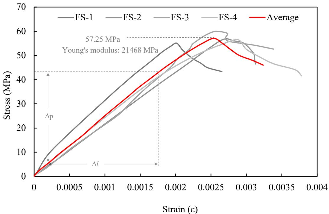
Figure 6. 31 Relationship between stress (MPa) and strain ( $\epsilon$ ) of treated wood (albasia Voronoi composite) in longitudinal direction compressive strength test.
