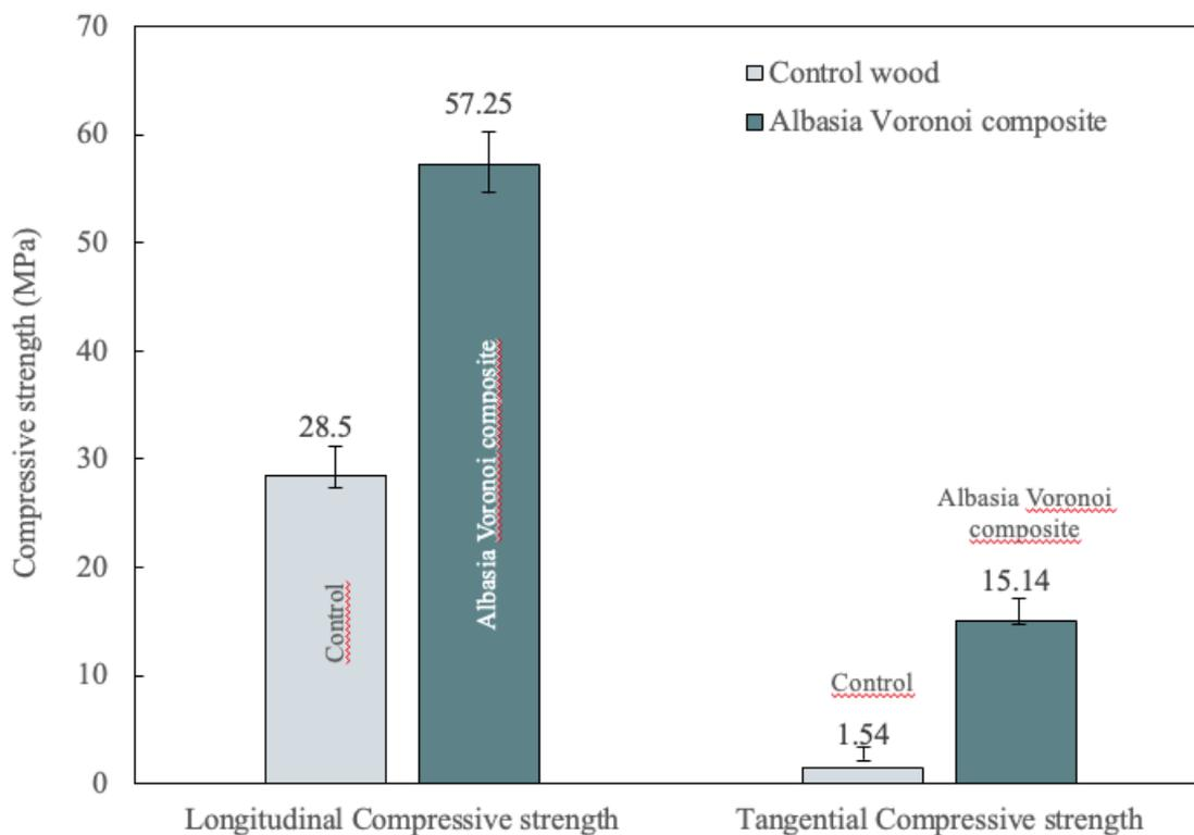
Figure 6. 45 Comparative analysis of compressive strength.
