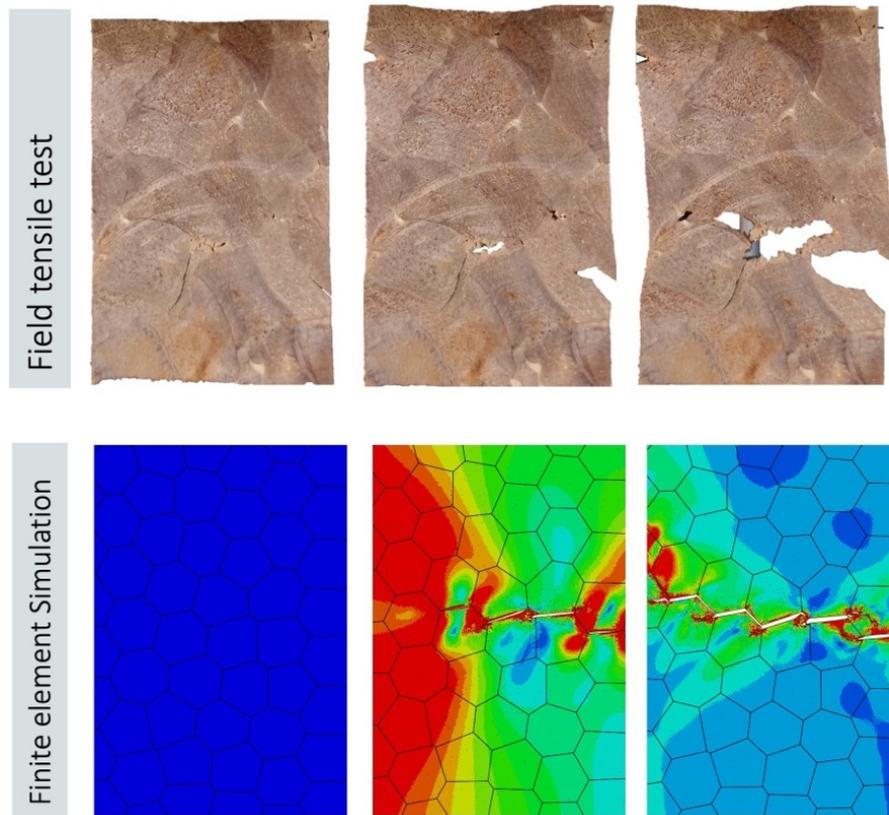
Figure 6. 59 Comparative study between field tensile test and FEM simulation
