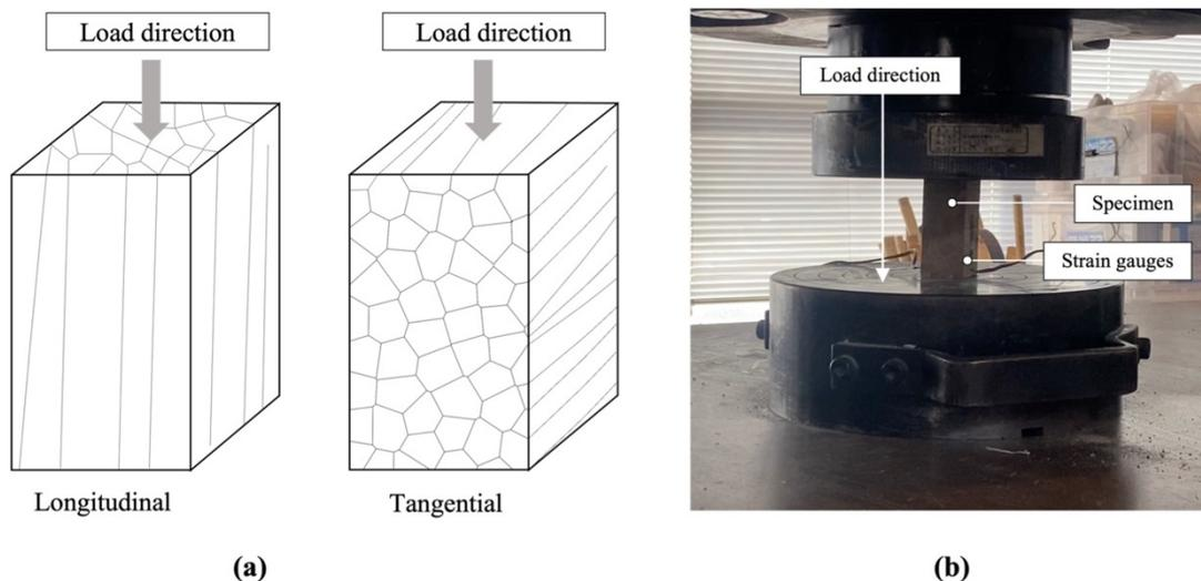
Figure 7. 10 Loading application of compressive strength test.
