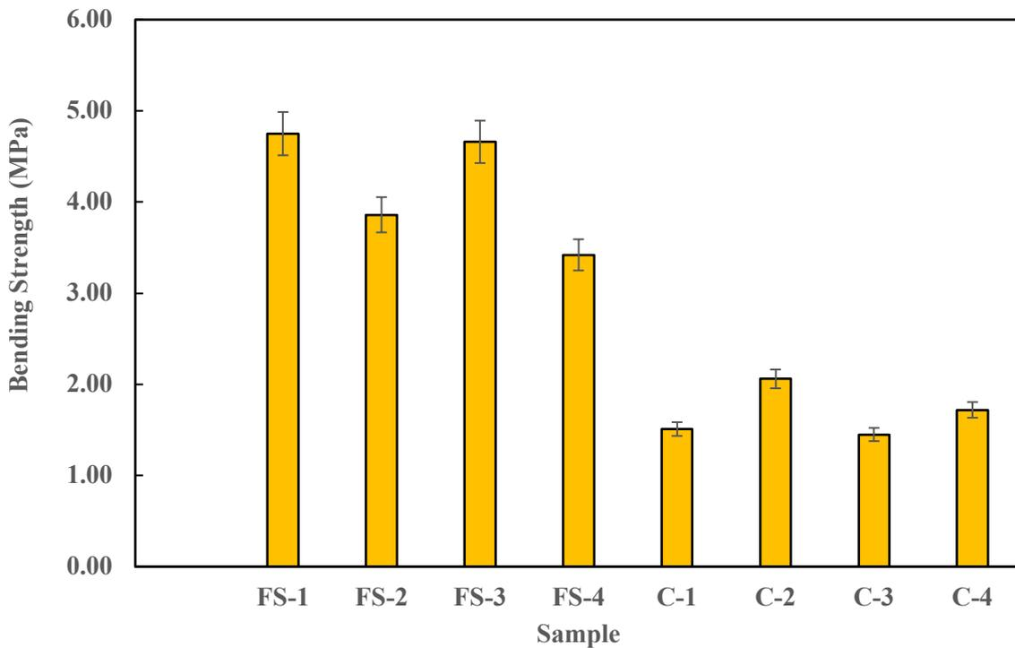
Figure 6. 49 Bending Strength of treated and control albasia wood.
