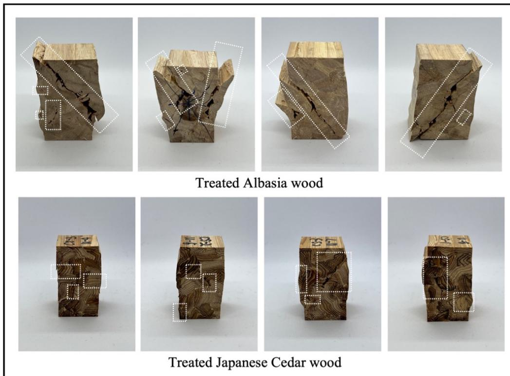
Figure 7. 19 Representative photographs of typical failure patterns of treated albasia and Japanese cedar wood tangential compression test.
