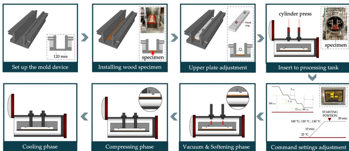
Figure 5. 1 Schematic illustration of the high-temperature and -pressure process.
