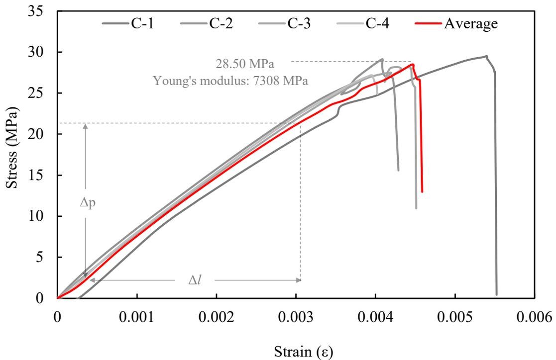
Figure 6. 32 Relationship between stress (MPa) and strain ( $\epsilon$ ) of control wood in longitudinal direction compressive strength test.
