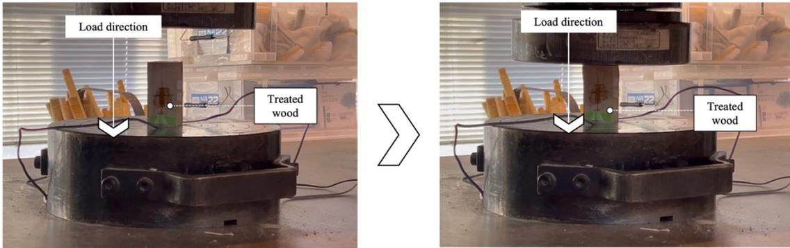
Figure 6. 30 Longitudinal compressive strength test on the treated wood
