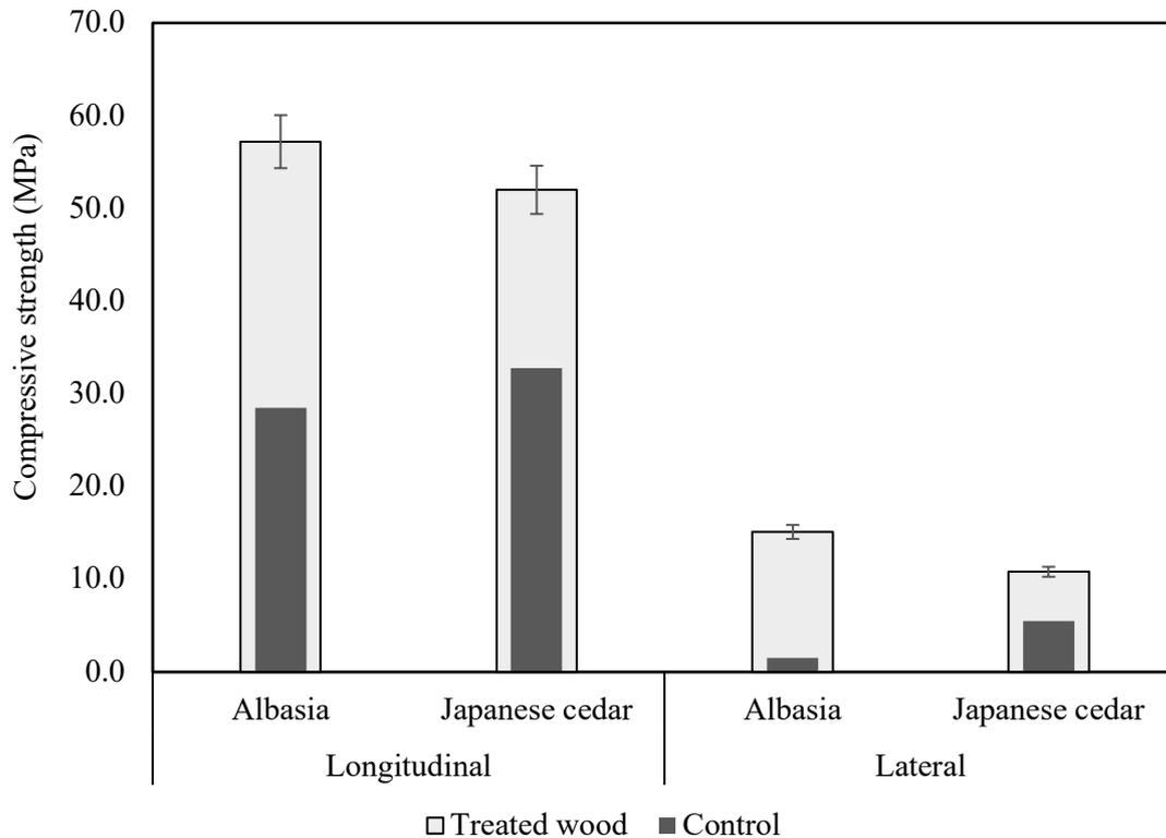
Figure 7. 22 Comparison of maximum compressive strength between control and treated albasia and Japanese cedar wood.
