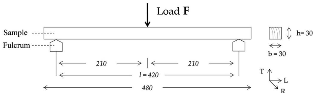
Figure 6. 15 Schematic Illustration for three-point longitudinal bending tests.
