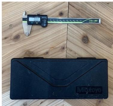
Figure 3. 13 a caliper with an accuracy of 0.01 mm (Mitutoyo: ABSOLUTE Digimatic Scale Units-572 Series 0-8in/0–200 mm)
