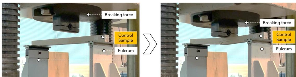
Figure 6. 46 Longitudinal bending strength test on control wood.
