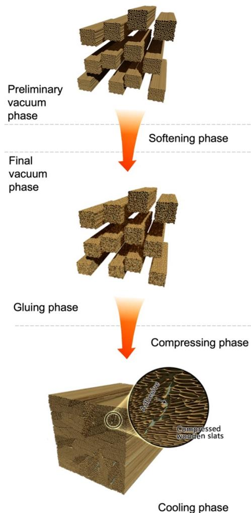
Figure 6. 10 Illustration of Albasia Voronoi Composite treatment.
