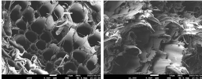
Figure 6. 27 SEM Micrographs of control (left) and treated (right) wood.
