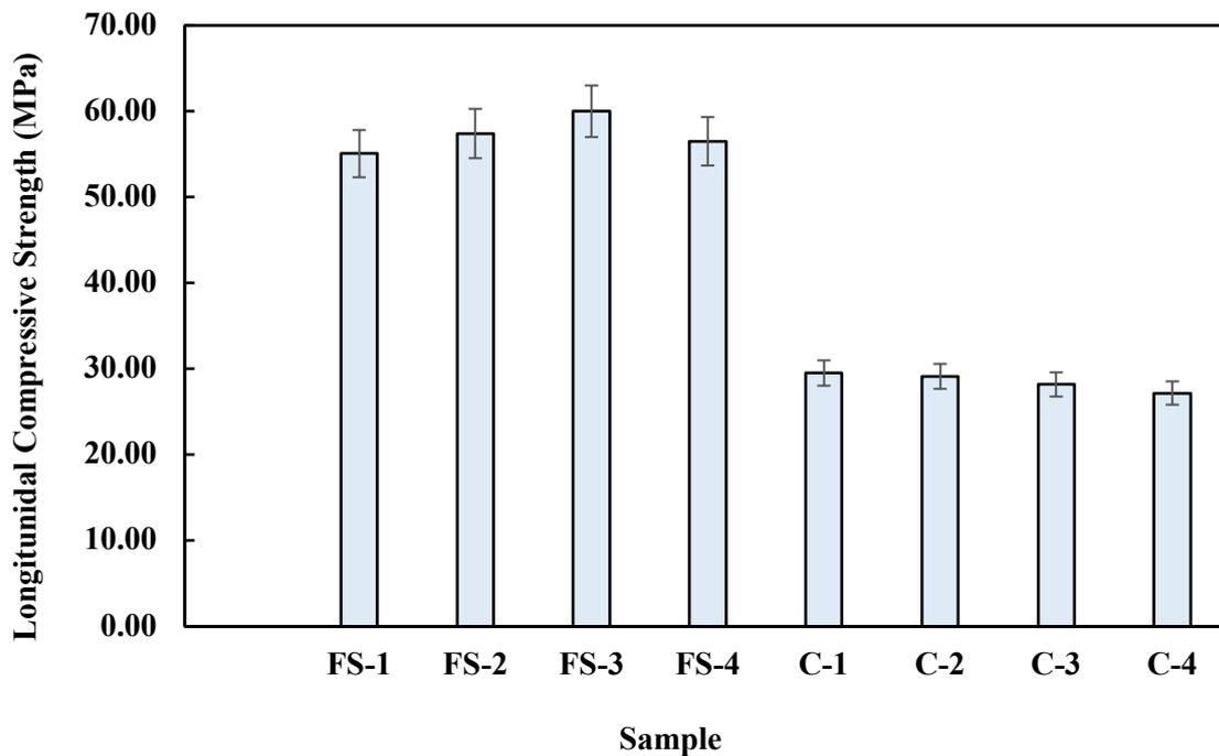
Figure 6. 36 Longitudinal Compressive Strength of treated and control albasia wood.
