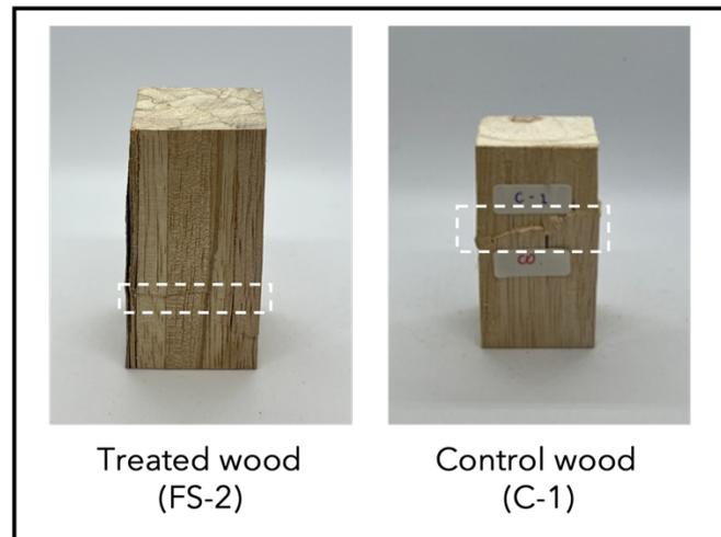
Figure 6. 35 Crushing failure type of wood in compressive strength test parallel to grain (longitudinal direction)
