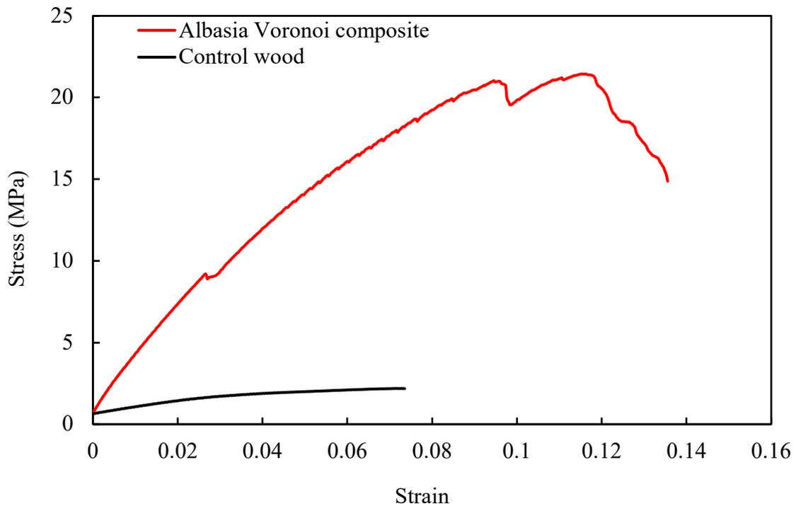
Figure 6. 52 Comparative relationship between stress (MPa) and strain ( $\epsilon$ ).
