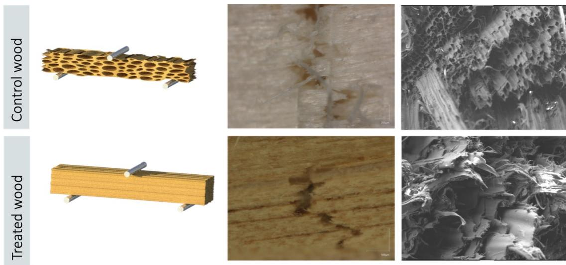
Figure 6. 50 Observation of the microscopic scale on bending strength test.
