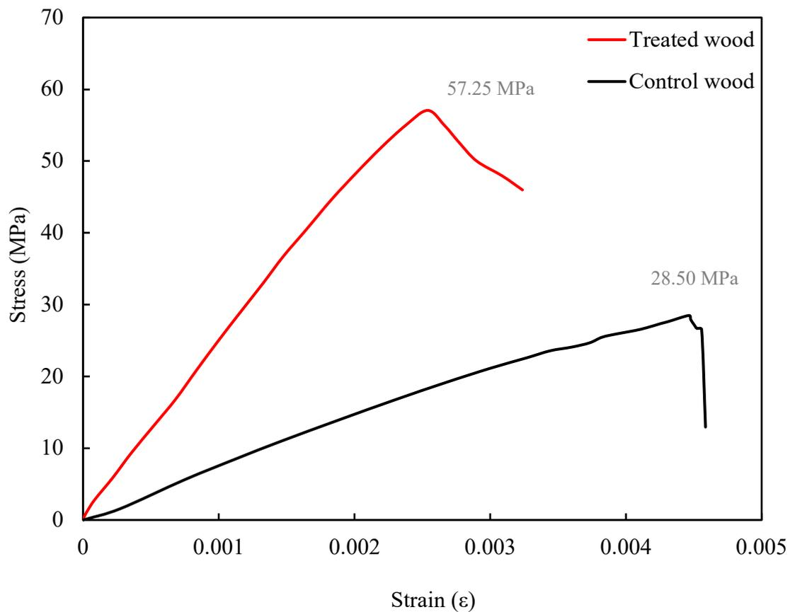
Figure 6. 33 Comparative relationship between stress (MPa) and strain ( $\epsilon$ ) of treated and control wood in longitudinal direction compressive strength test.
