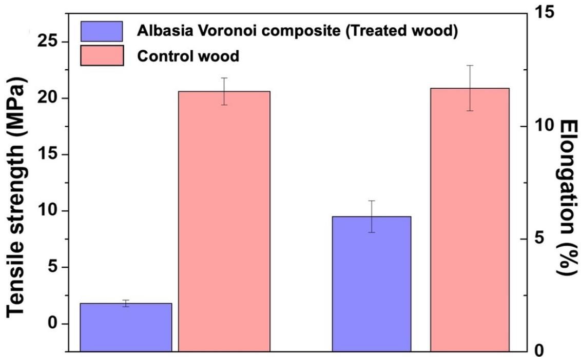
Figure 6. 55 The tensile strength (Mpa) and elongation (%) between treated wood and control wood along tangential direction.
