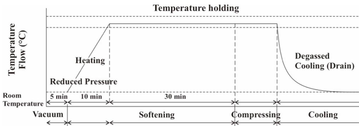
Figure 5. 2 Consolidation process on high-temperature and -pressure treatment.
