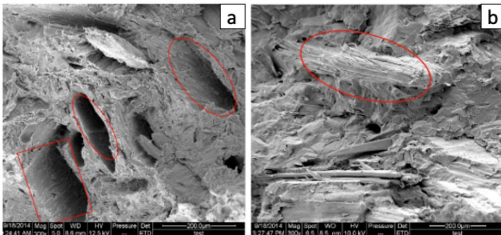
Figure 2. 6 SEM micrographs results of untreated (a) and treated wood (b)
