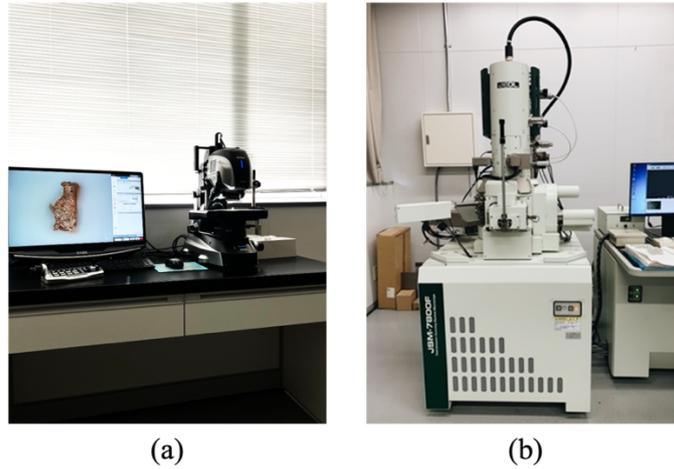
Figure 6. 12 (a) Digital Microscope: VHX-7000 series (b) Scanning Electron Microscopy: FE-SEM JSM-7800F
