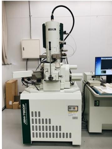
Figure 3. 17 Scanning Electron Microscopy: FE-SEM JSM-7800F.
