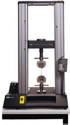
Figure 3. 24 Strain-controlled testing machine (Instron 5565 A) for tensile test
