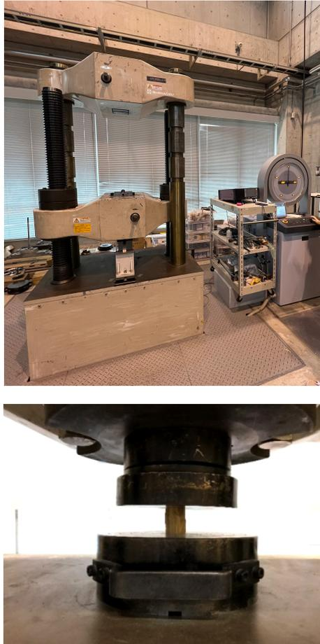
Figure 3. 19 Universal material testing machine UH-2000kNXR for compressive strength test.
