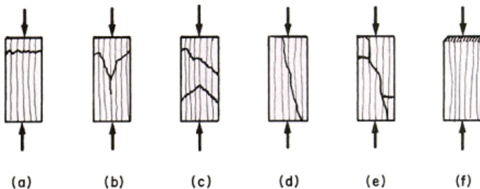
Figure 6. 34 Failure types of wood in compressive strength test parallel to grain (a) crushing, (b) wedge splitting, (c) shearing, (d) splitting, (e) crushing and splitting, (f) brooming or end rolling.
