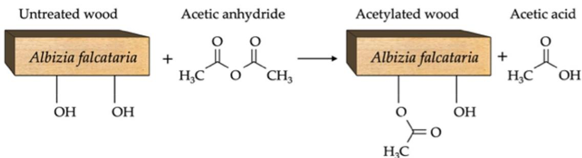
Figure 2. 9 Schematic view of the acetylation of Albisia.
