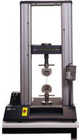
Figure 6. 17 Strain-controlled testing machine (Instron 5565 A) for tensile test
