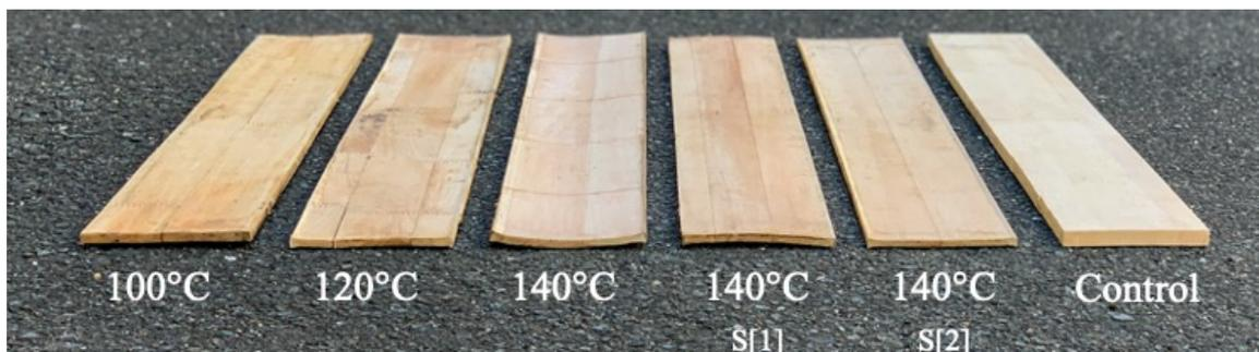
Figure 5. 8 Comparison of Albasia boards, both treated and control.
