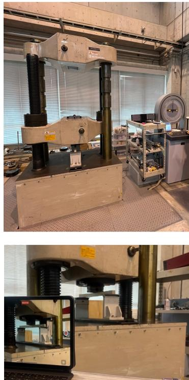
Figure 3. 21 Universal material testing machine UH-2000kNXR for bending strength test.
