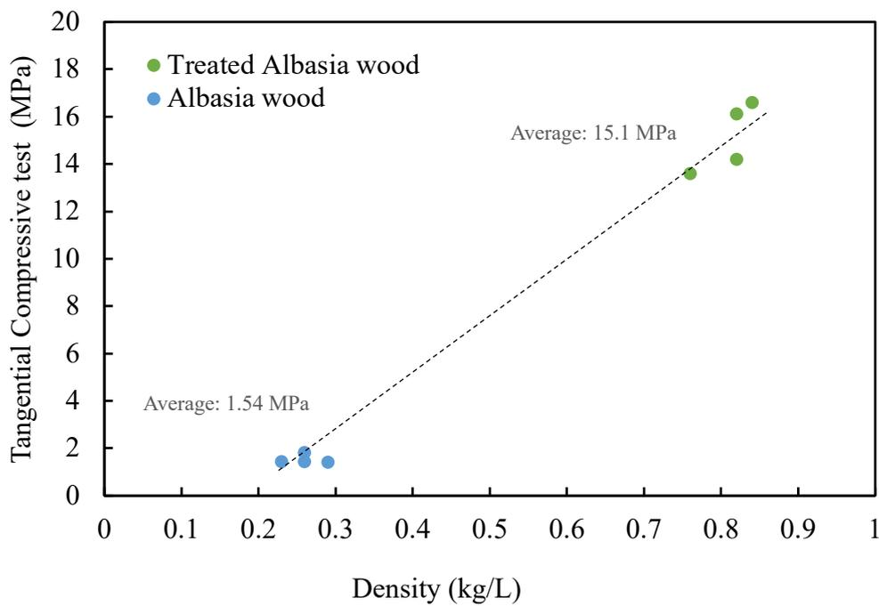
Figure 7. 20 Correlation between specific gravity and tangential compressive strength of treated and untreated albasia wood.
