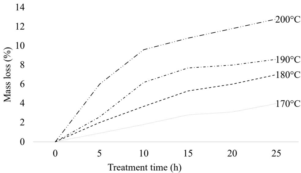
Figure 2. 5 The relationship between the mass loss of wood and the treatment time for the different temperature settings
