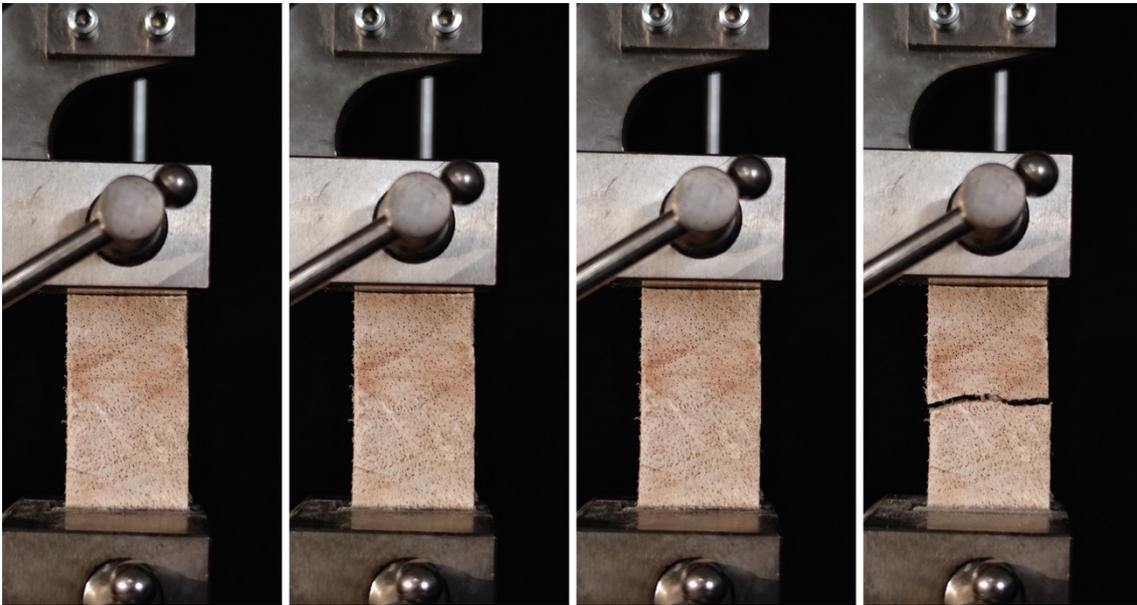
Figure 6. 56 Tensile test on control wood
