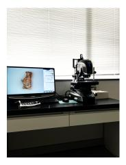
Figure 3. 16 Digital Microscope: VHX-7000 series.
