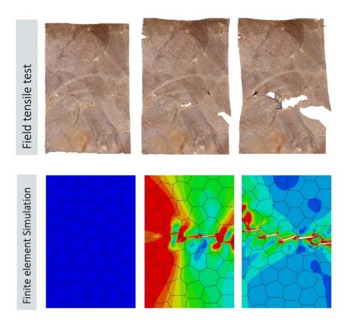
Figure 6. 59 Comparative study between field tensile test and FEM simulation
