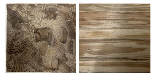
Figure 7. 14 Treated Japanese cedar wood (Left: Cross section); (Right: Fiber direction).
