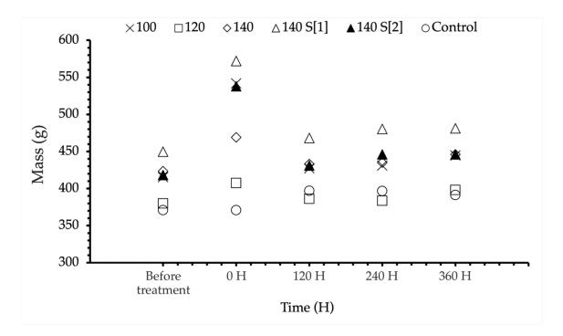
Figure 5. 5 Mass change of specimens.
