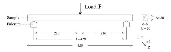
Figure 6. 15 Schematic Illustration for three-point longitudinal bending tests. Dimensions are presented in mm.
