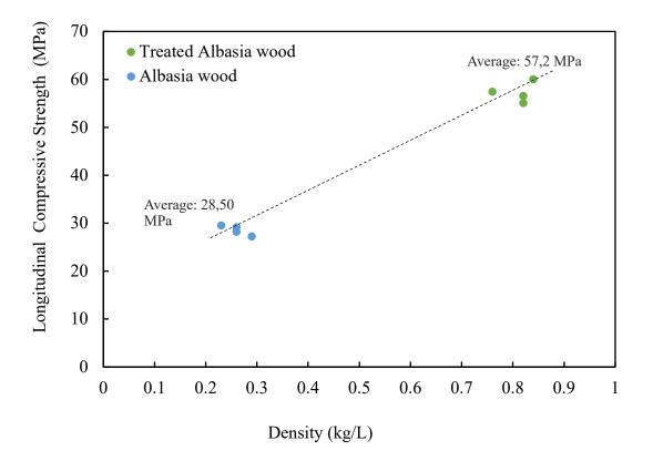
Figure 7. 17 Correlation between specific gravity and longitudinal compressive strength of treated and untreated albasia.
