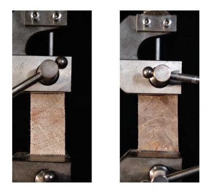
Figure 6. 18 Tensile test on control wood (left) and treated wood (right).
