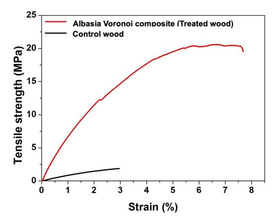
Figure 6. 54 Relationship curves between tensile stress and strain of control and treated wood (albasia Voronoi composite).
