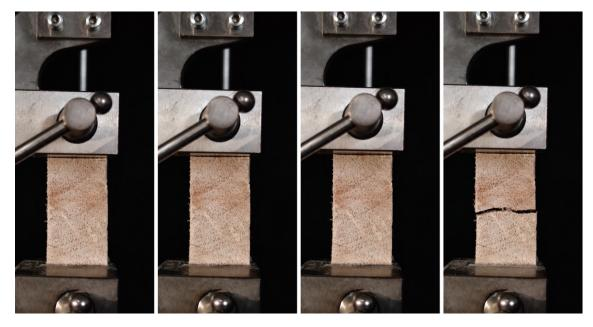
Figure 6. 56 Tensile test on control wood
