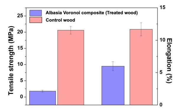
Figure 6. 55 The tensile strength (Mpa) and elongation (%) between treated wood and control wood along tangential direction.
