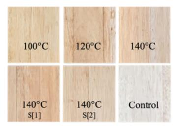
Figure 5. 7 Color differences of albasia wood at different temperatures and pressures.
