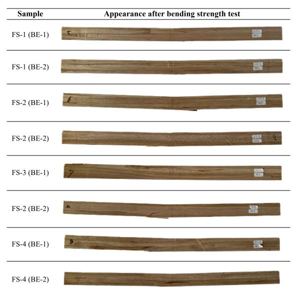
Table 6. 14 Appearance of treated samples after bending strength test
