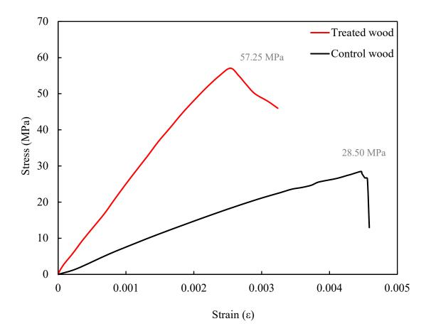
Figure 6. 33 Comparative relationship between stress (MPa) and strain (ε) of treated and control wood in longitudinal direction compressive strength test.
