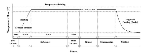
Figure 6. 8 Consolidation process of Albasia Voronoi composite wood.
