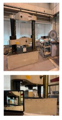
Figure 3. 21 Universal material testing machine UH-2000kNXR for bending strength test.
