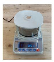
Figure 3. 14 Digital scale with an accuracy of 0.01 g (A&D: FZ-5000i)
