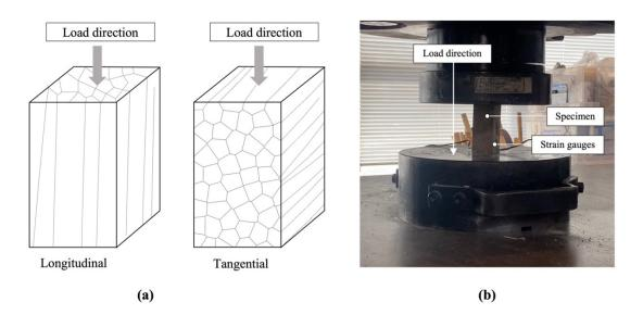
Figure 7. 10 Loading application of compressive strength test.
