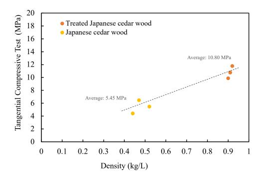
Figure 7. 21 Correlation between specific gravity and tangential compressive strength of treated and untreated Japanese cedar wood.
