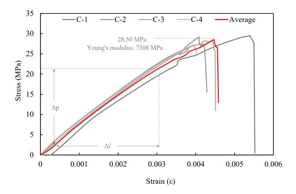
Figure 6. 32 Relationship between stress (MPa) and strain (ε) of control wood in longitudinal direction compressive strength test.
