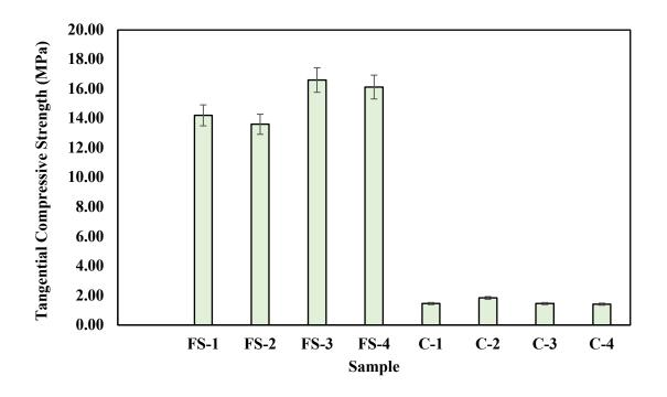
Figure 6. 44 Tangential Compressive Strength of treated and control albasia wood
