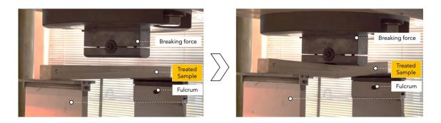
Figure 6. 47 Longitudinal bending strength test on treated wood.
