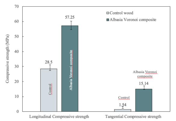
Figure 6. 45 Comparative analysis of compressive strength.
