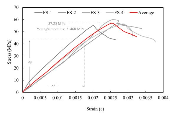
Figure 6. 31 Relationship between stress (MPa) and strain (ε) of treated wood (albasia Voronoi composite) in longitudinal direction compressive strength test.
