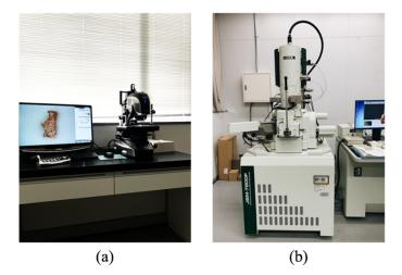
Figure 6. 12 (a) Digital Microscope: VHX-7000 series (b) Scanning Electron Microscopy: FE-SEM JSM-7800F
