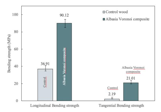
Figure 6. 53 Comparative analysis of bending strength.
