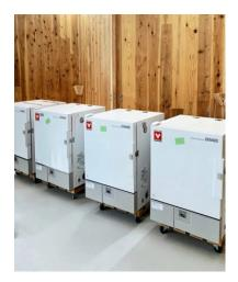
Figure 3. 18 Constant oven DKM600 for drying sample.
