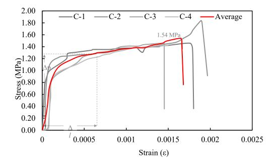
Figure 6. 40 Relationship between stress (MPa) and strain (ε) of control wood in tangential direction compressive strength.
