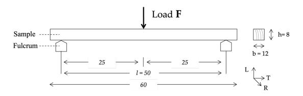
Figure 6. 16 Schematic Illustration for three-point tangential bending tests. Dimensions are presented in mm.
