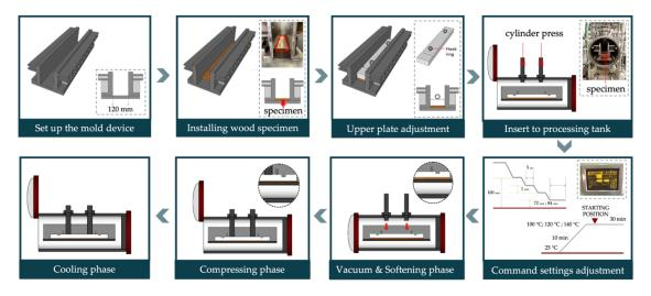
Figure 5. 1 Schematic illustration of the high-temperature and -pressure process.
