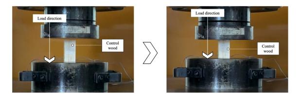
Figure 6. 29 Longitudinal compressive strength test on the control wood
