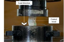
Figure 6. 37 Tangential compressive strength test on the control wood
