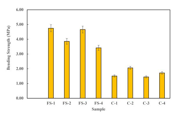
Figure 6. 49 Bending Strength of treated and control albasia wood.
