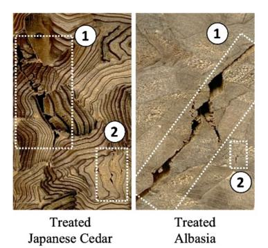
Figure 7. 23 A close-up view of cracks and fractures in the specimen after compressive strength test.
