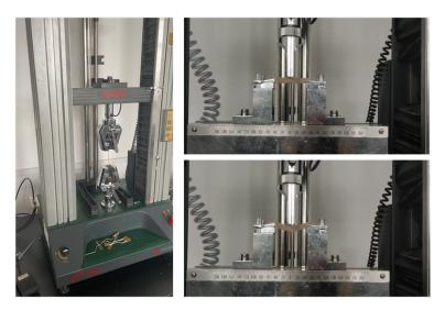
Figure 3. 23 Universal material testing machine CMT6104 for bending strength test.
