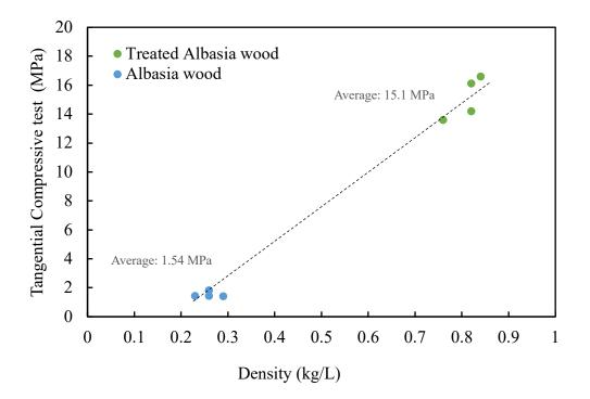
Figure 7. 20 Correlation between specific gravity and tangential compressive strength of treated and untreated albasia wood.
