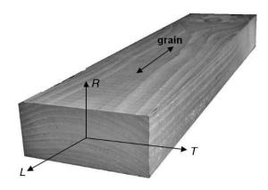
Figure 2. 3 Orthotropic directions for wood properties
