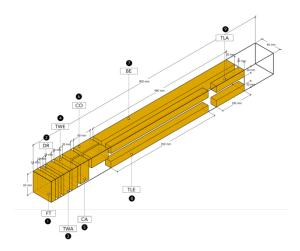
Figure 6. 11 Wood cutting pattern on treated sample.
