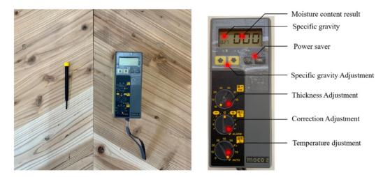
Figure 3. 15 Wood moisture content meter (Kett: HM-530 20 MHz / range 2-50%)
