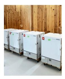
Figure 6. 13 Constant oven DKM600 for drying sample.
