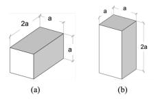
Figure 3. 20 The dimension of a wood sample for the compressive strength
