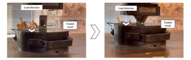
Figure 6. 38 Tangential compressive strength test on the treated wood (albasia Voronoi composite)
