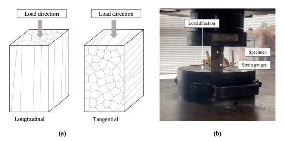
Figure 6. 14 Loading application of compressive strength test.
