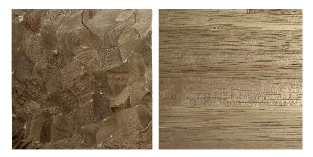
Figure 7. 13 Treated albasia wood (Left: Cross section); (Right: Fiber direction).
