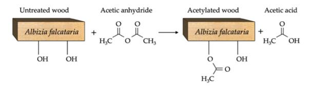
Figure 2. 9 Schematic view of the acetylation of Albasia.
