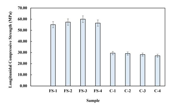
Figure 6. 36 Longitudinal Compressive Strength of treated and control albasia wood.
