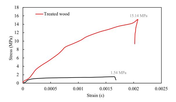
Figure 6. 41 Comparative relationship between stress (MPa) and strain (ε) of treated and control wood in tangential direction compressive strength test.
