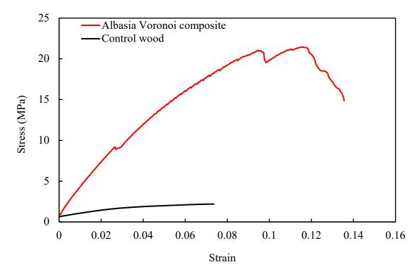
Figure 6. 52 Comparative relationship between stress (MPa) and strain  $(\varepsilon)$ .
