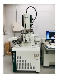
Figure 3. 17 Scanning Electron Microscopy: FE-SEM JSM-7800F.
