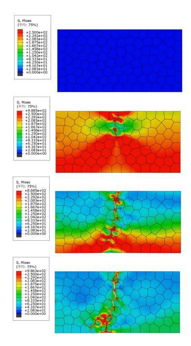
Figure 6. 58 Finite Element Model (FEM) Simulation on treated wood
