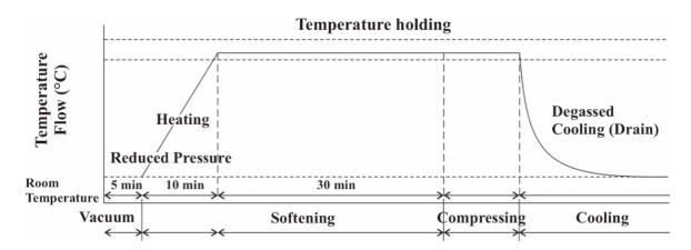
Figure 5. 2 Consolidation process on high-temperature and -pressure treatment.
