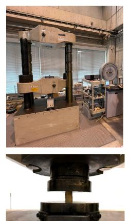
Figure 3. 19 Universal material testing machine UH-2000kNXR for compressive strength test.
