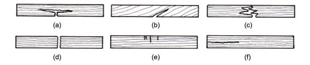
Figure 6. 48 Failure types of clear wood in bending with span parallel to grain: (a) simple tension, (b) cross-grain tension, (c) splintering tension, (d) brash tension, (e) compression, (f) horizontal shear.
