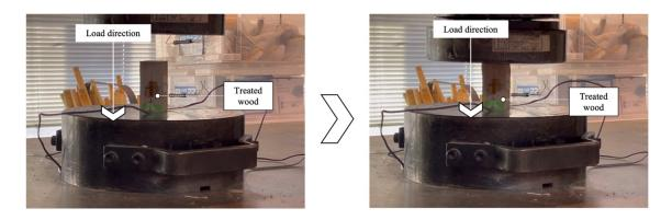
Figure 6. 30 Longitudinal compressive strength test on the treated wood
