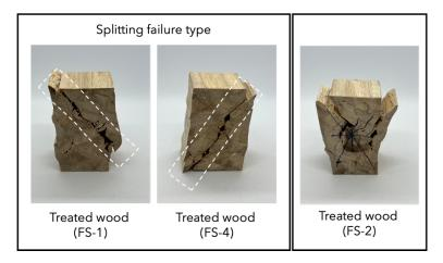
Figure 6. 42 Splitting failure type of wood in compressive strength test tangential direction on treated wood (albasia Voronoi composite)
