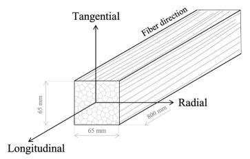
Figure 7. 12 Shape and dimensions of the specimens.
