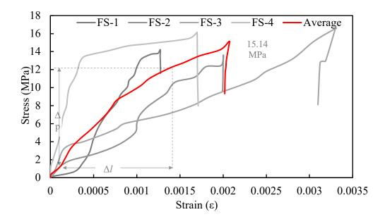
Figure 6. 39 Relationship between stress (MPa) and strain (ε) of of treated wood (albasia Voronoi composite) in tangential direction compressive strength.
