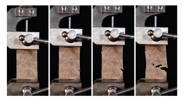
Figure 6. 57 Tensile test on treated wood.
