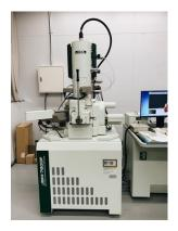
Figure 5. 3 SEM Investigation equipment: FE-SEM JSM-7800F
