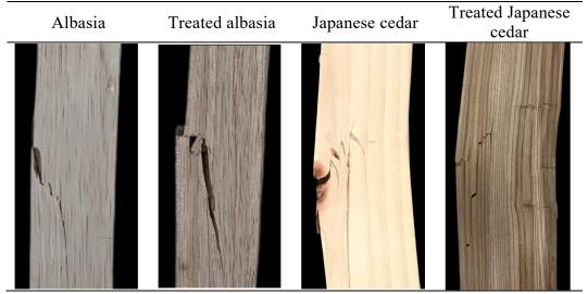
Table 7. 6 Typical failure pattern after bending strength test.
