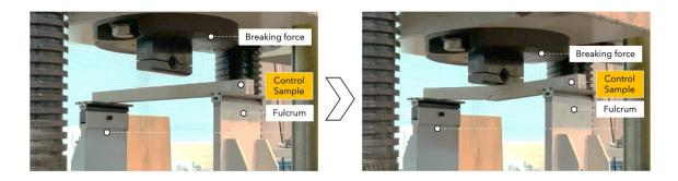
Figure 6. 46 Longitudinal bending strength test on control wood.
