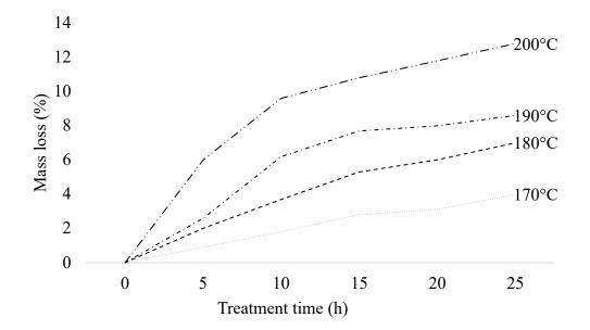
Figure 2. 5 The relationship between the mass loss of wood and the treatment time for the different temperature settings
