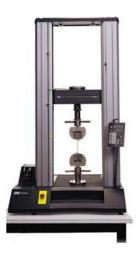
Figure 6. 17 Strain-controlled testing machine (Instron 5565 A) for tensile test Source: Instron Company, America (https://www.instron.com/en-gb/)
