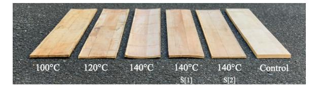
Figure 5. 8 Comparison of Albasia boards, both treated and control.
