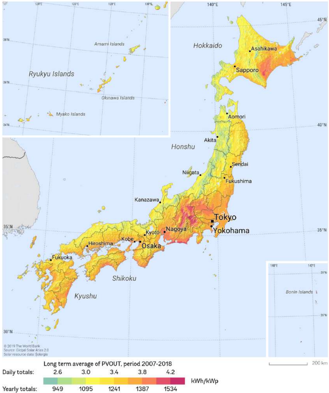
Fig 3. 3 Photovoltaic power potential in Japan [1] (The maps and data for Japan have been released in parallel with Global Solar Atlas, which is published by the World Bank Group, funded by ESMAP, and prepared by Solargis. All maps on this page are licensed by The World Bank under the Creative Commons Attribution license (CC BY 4.0) with the mandatory and binding addition presented in Global Solar Atlas terms. You are free to download, share, adapt, use the maps but you must give appropriate attribution:2020 The World Bank, Source: Global Solar Atlas 2.0, Solar resource data: Solargis.)
