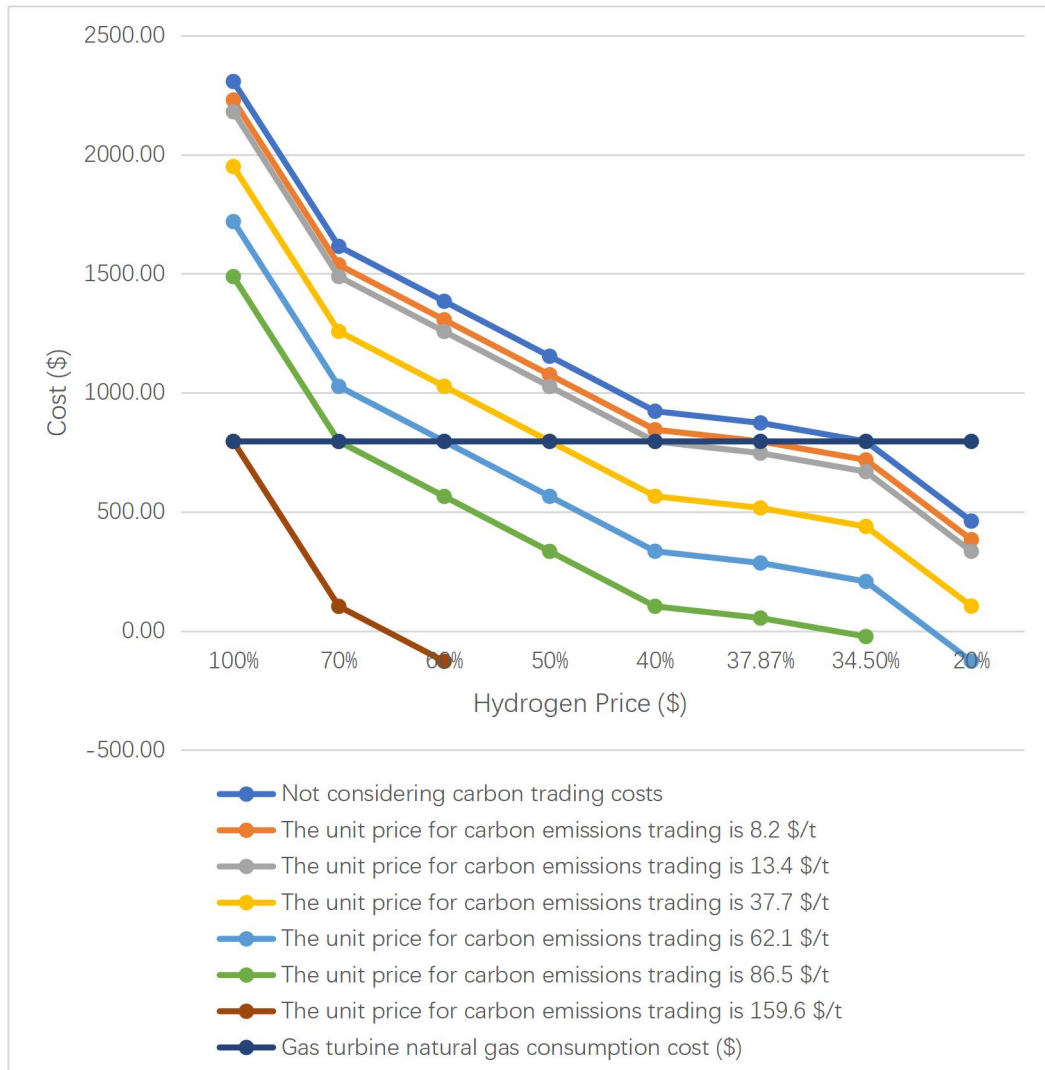
Fig.6-8 Changes in fuel consumption costs with different hydrogen blending ratios under different carbon emission trading unit prices
