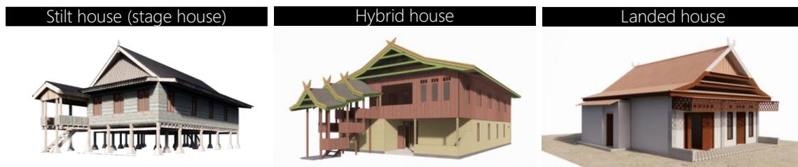
Figure 5.6 Examples of house types based on the structure type
