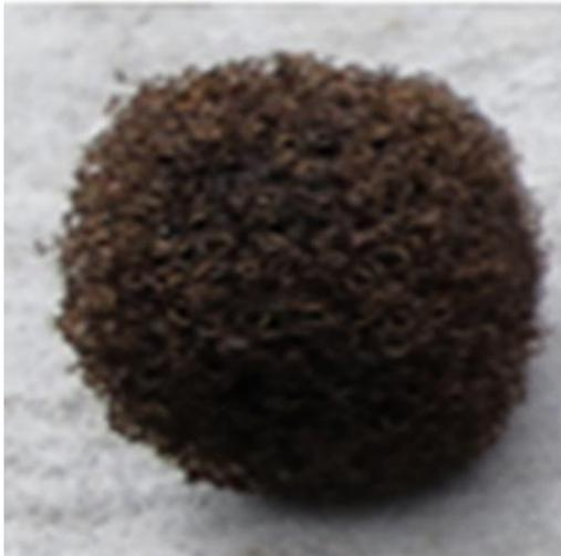
**Figure 2.11.** Photo of a sponge carrier media obtained from Seki wastewater treatment plant, Gifu prefecture, Japan.
