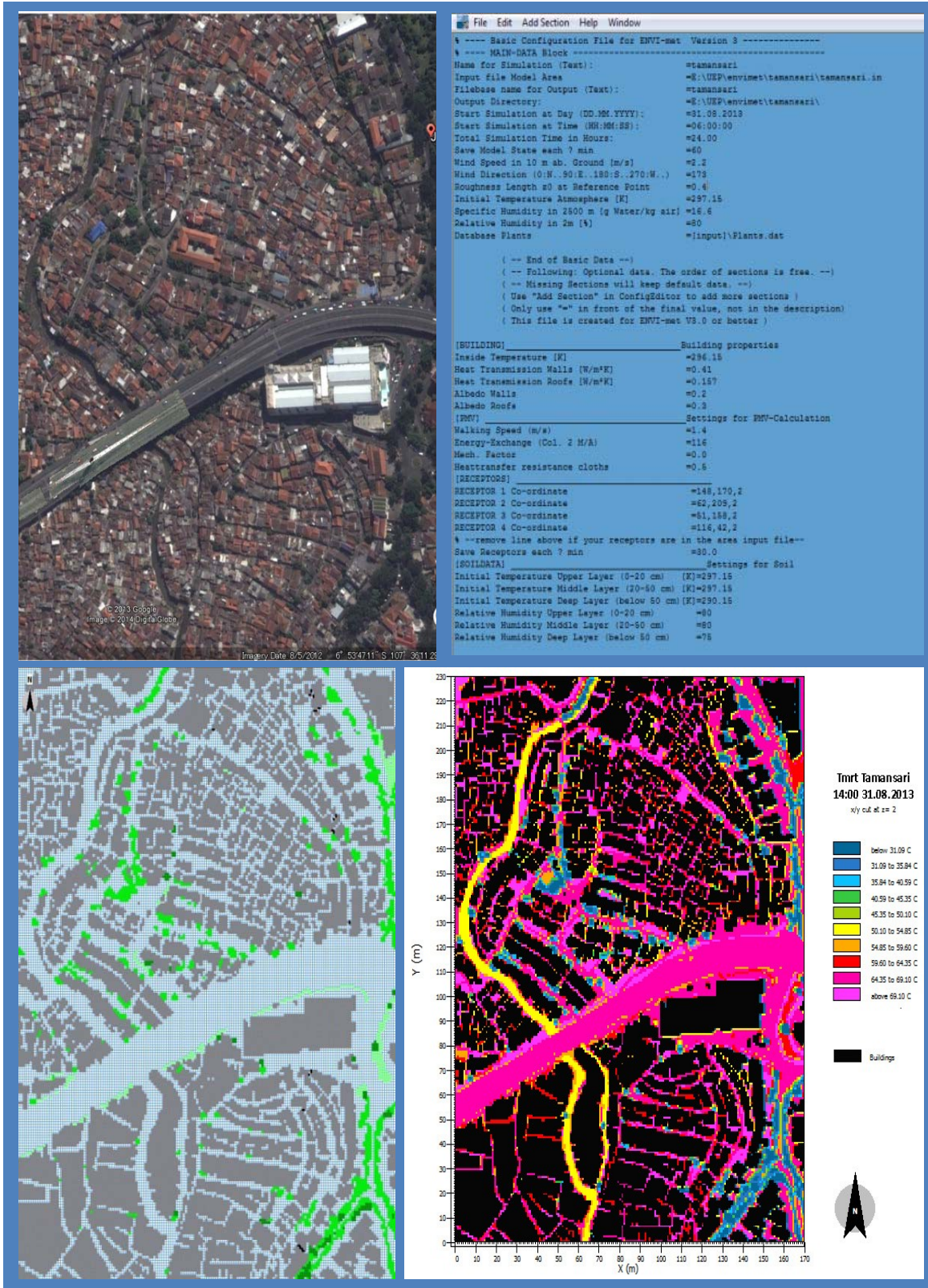
Fig. 6.1 (a) Tamansari in satellite image; (b) configuration input; (c) ENVI-met model; (d) Tmrt visualization of ENVI-met at the hottest time
