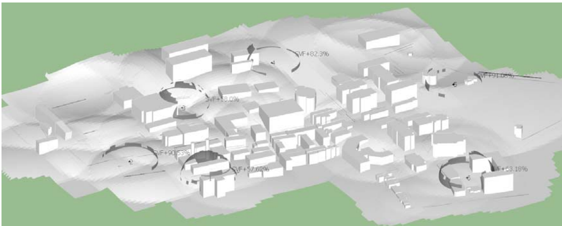
Fig. 5.6. Urban Form and Sky View Factor of UPI-Educational. Source: Modeled by Sketch-up, SVF generated by Chronolux, author
