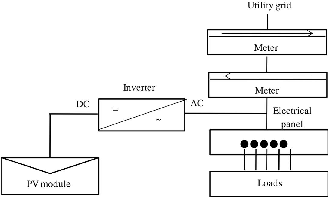
Fig. 6-2 Schematic of grid-connected PV system
