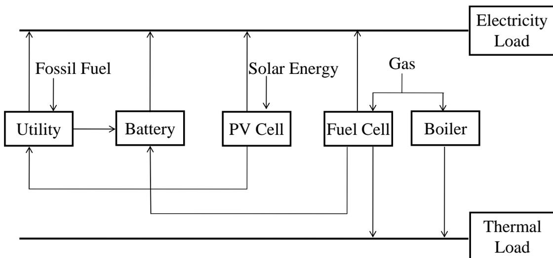
**Fig. 7-1 Energy flow of the hybrid PV/CHP/battery system**
