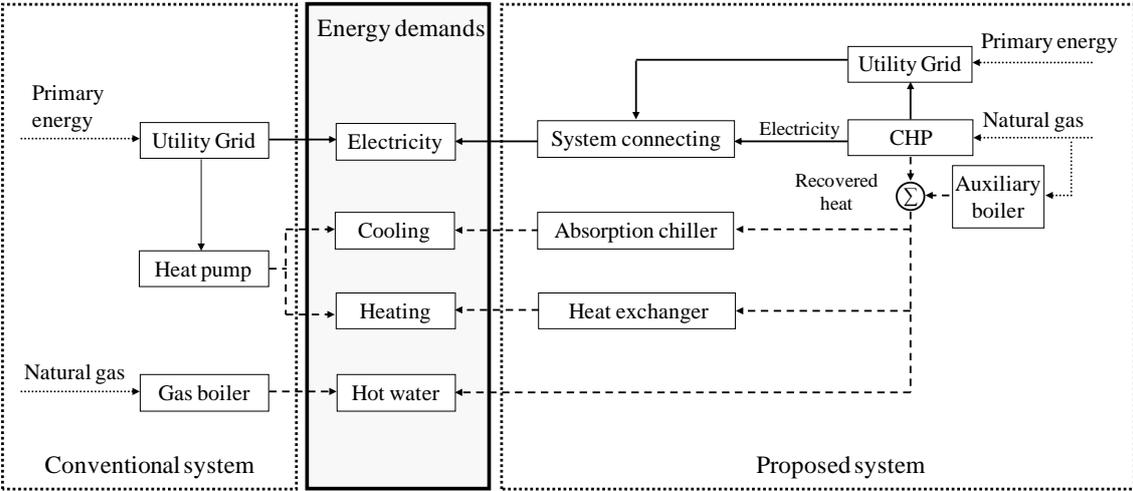
**Fig. 5-2 Super structure of the conventional system and the proposed system**
