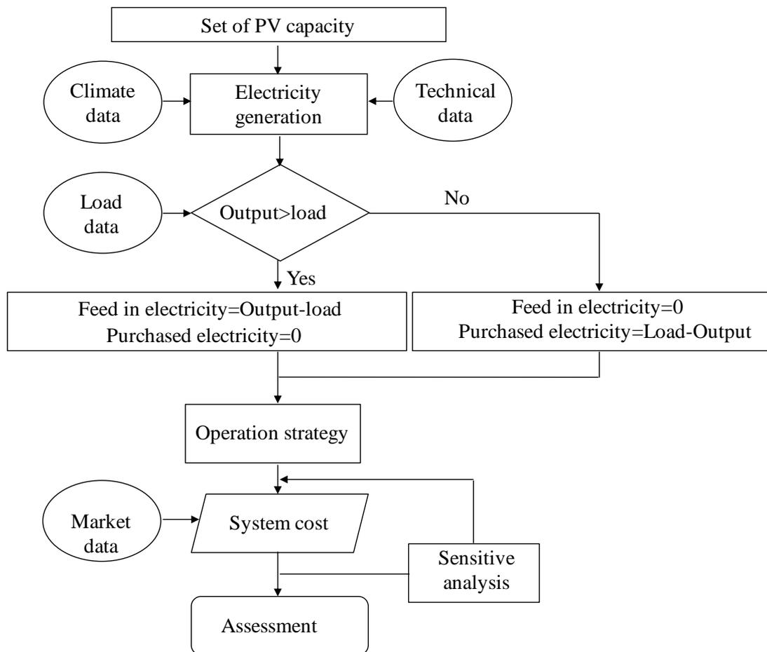
**Fig. 6-3** The algorithm of PV system analysis procedure
