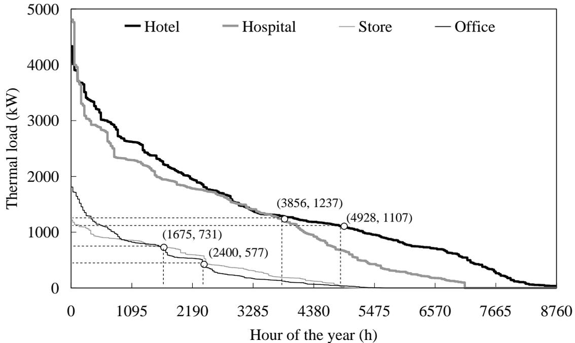
**Fig. 5-5 Thermal load duration curves for various buildings in Tokyo**
