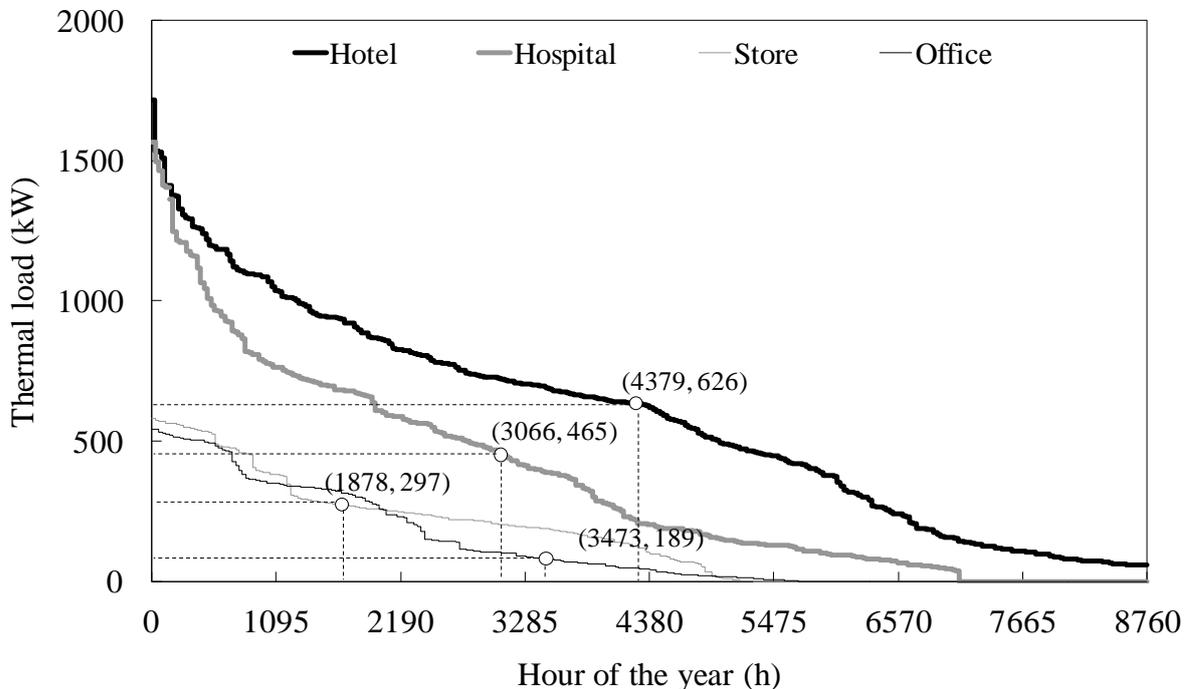
Fig. 5-11 Thermal load duration curves for various buildings in Shanghai
