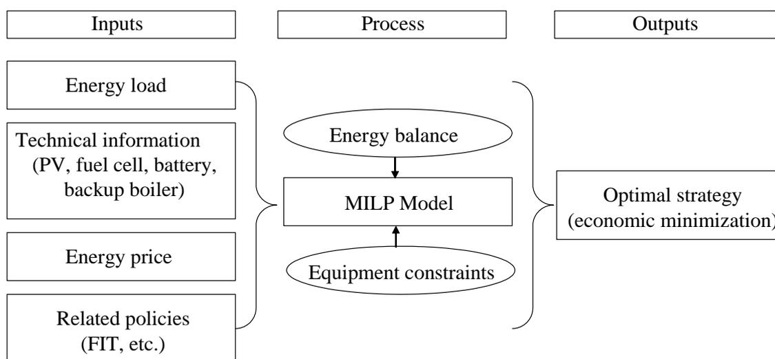
**Fig. 4-1 Flow chart of the optimization model**
