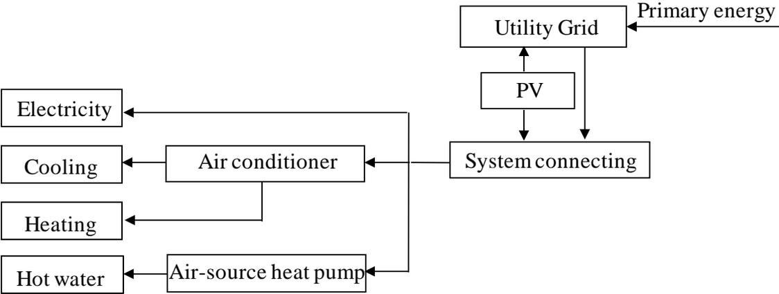
Fig. 6-1 Block diagram of PV system
