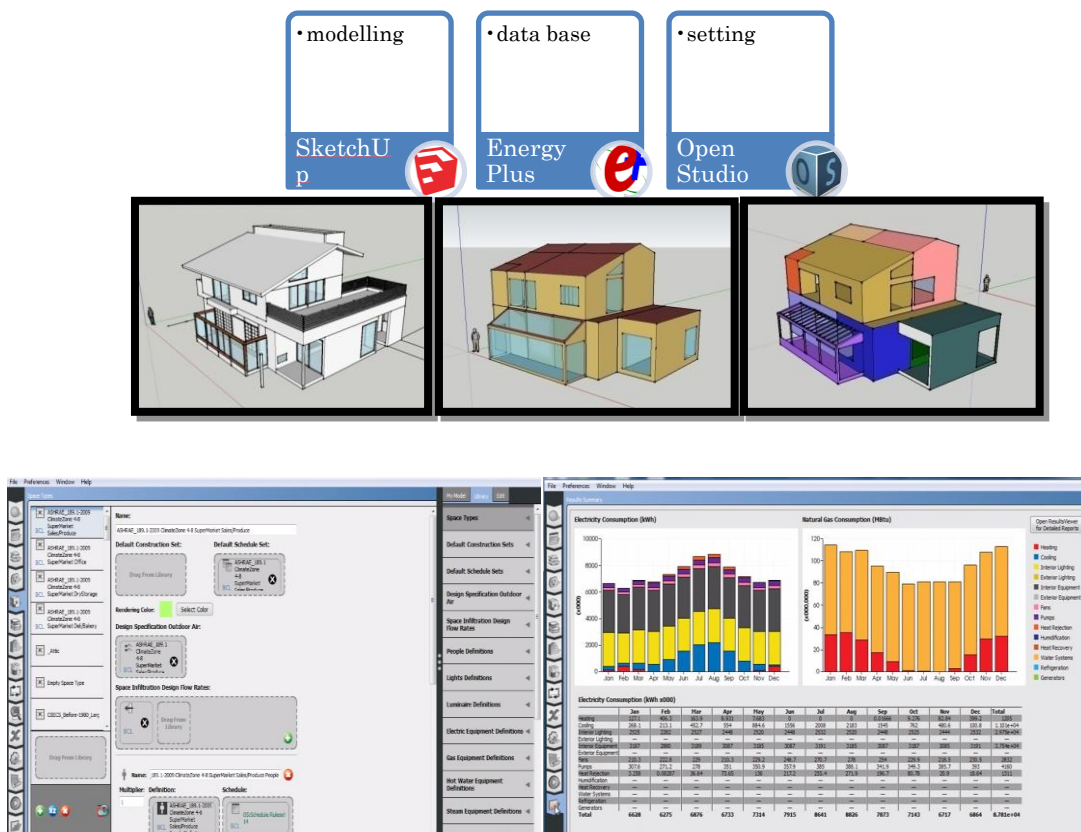
Figure 2-3 Display in sketch-up with energy-plus and open studio software
