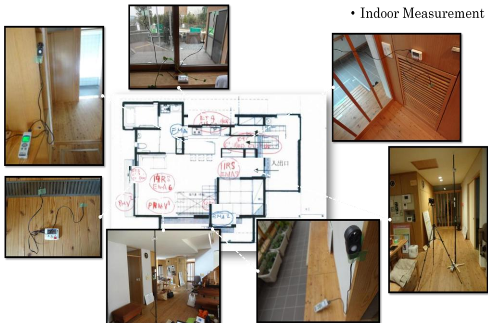
Figure 6-8 The installation of thermal environment measurement tools
