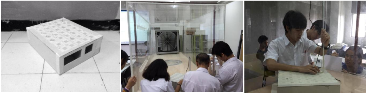
Figure 5.2 Testing airflow speed of two-bedroom type of Klong Chan Flat, Faculty of Architecture, Rajamangala University of Technology Thanyaburi (RMUTT), 2015
