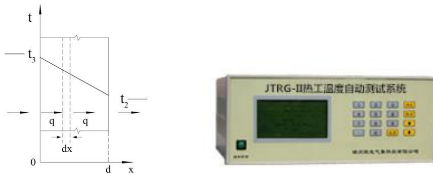
(a) One-dimensional-steady-state heat transfer principle (b) Measuring instrument
