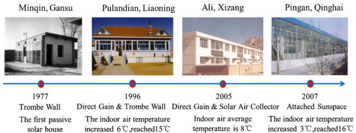
Fig.1-3 Development of passive solar house in China[45]
