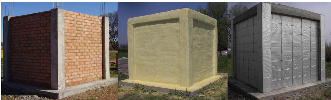
Figure 1-15 Comparison cubicles: brick cubicle, brick cubicle with polyurethane, brick cubic with RT-27 and polyurethane[14]
