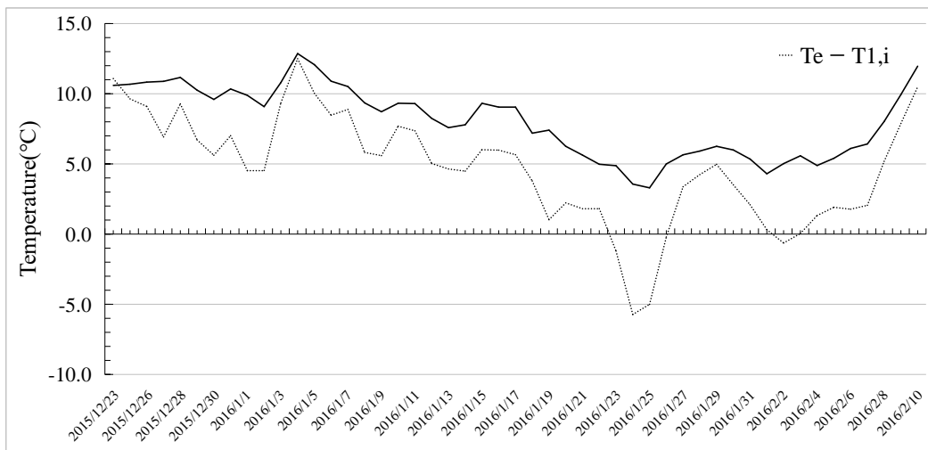
Fig.5- 4. Comparison of daily mean indoor temperature \overline{T_{1,i}} and mean outdoor temperature \overline{T_e} ( 23 rd December 2015 to 10 th February 2016 )
