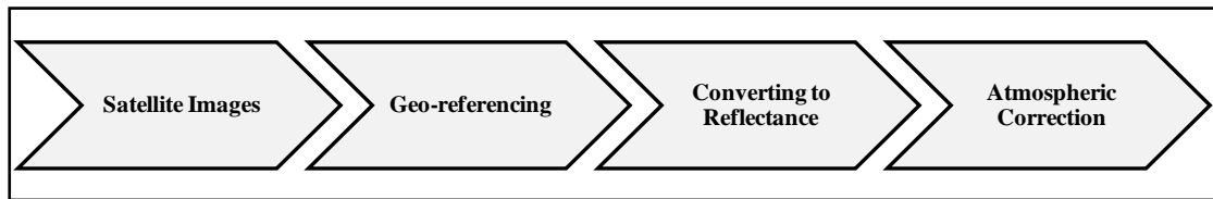
Figure 5-2 Pre-processing steps of Landsat TM and OLI images
