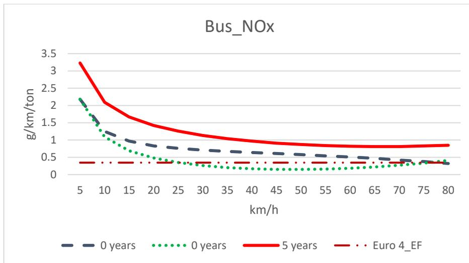
Figure 3.11 Emission factor measurement of bus\_NOx
