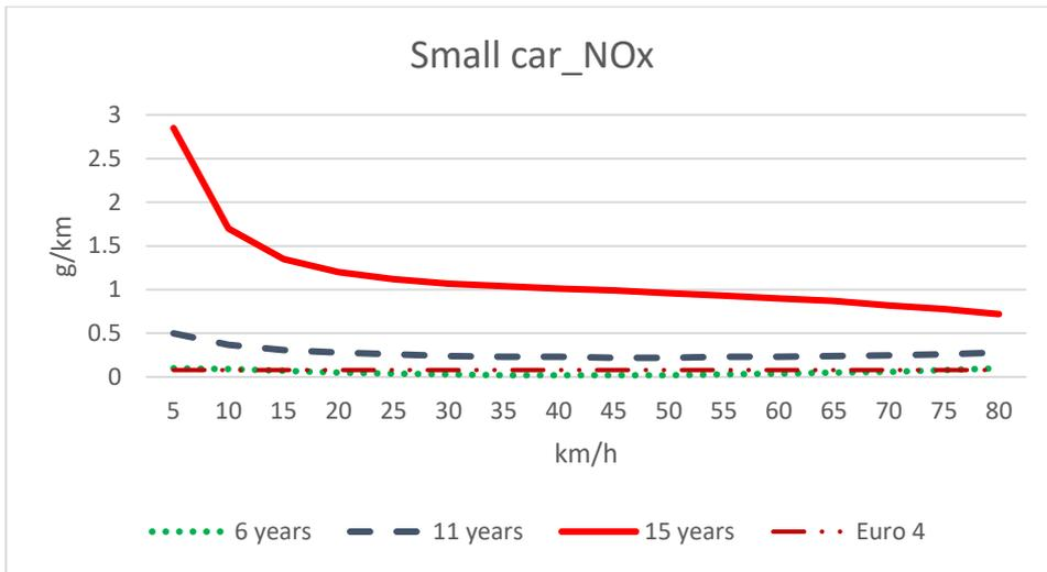
Figure 3.8 Emission factor measurement of small car
