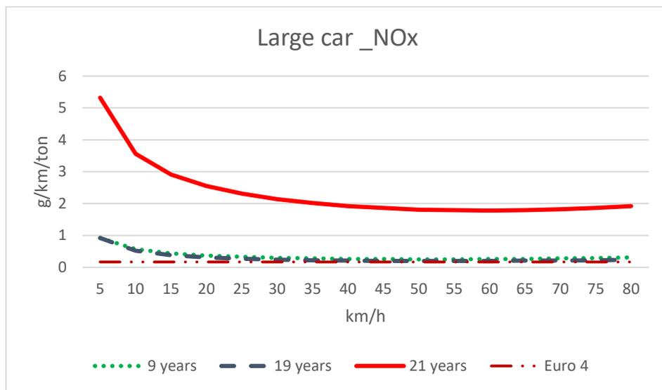
Figure 3.9 Emission factor measurement of large car\_NOx
