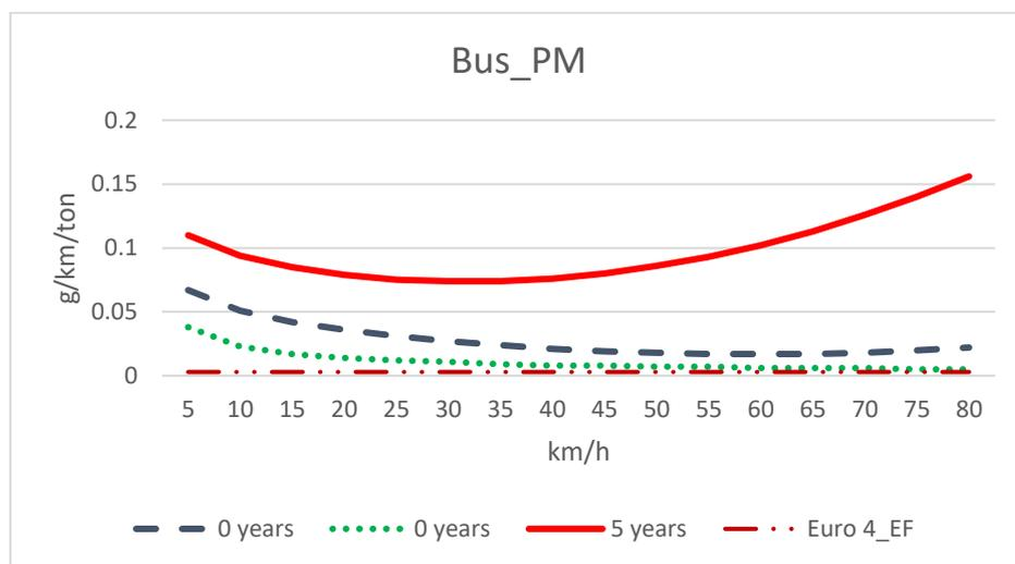
Figure 3.12 Emission factor measurement of bus\_PM
