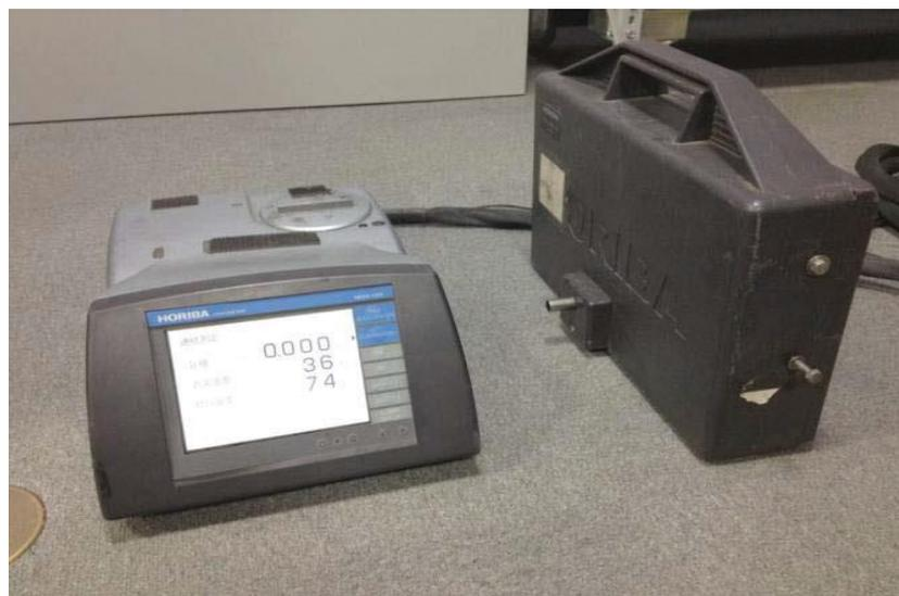
Figure 5.7 MEXA-130S PM analyzer
