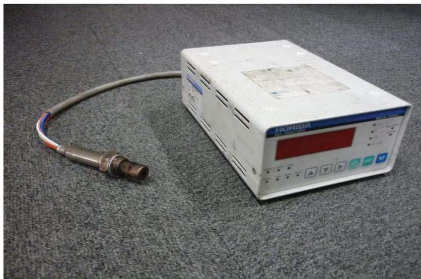
Figure 5.6 MEXA-720 NO<sub>x</sub> analyzer
