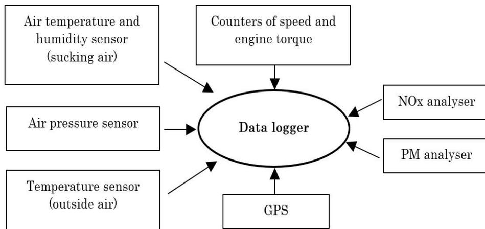
Figure 5.5 On-board emission measurement system scheme
