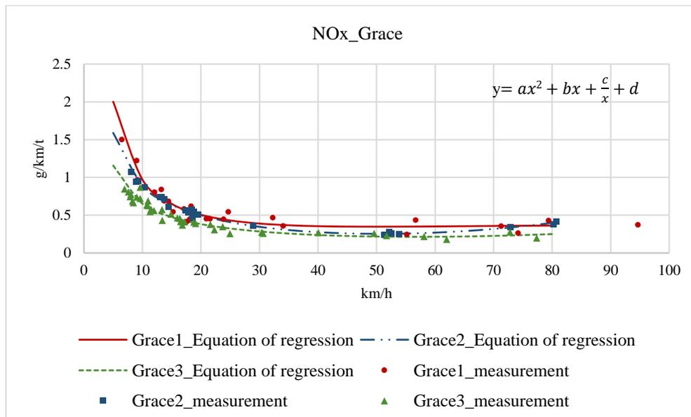
Figure 5.9 EF of NO<sub>x</sub> vehicle with diesel engine
