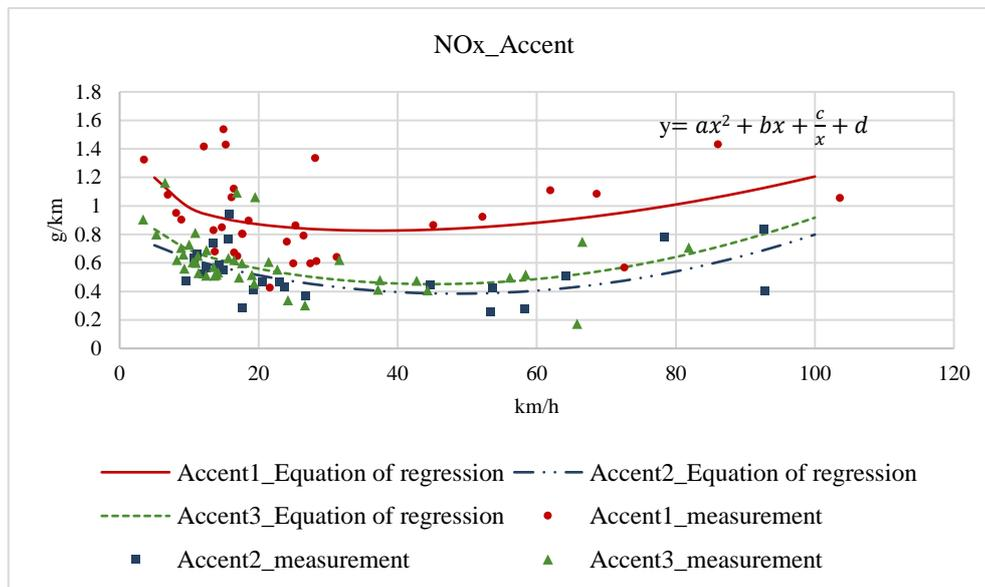
Figure 5.8 EF of NO<sub>x</sub> vehicle with gasoline engine
