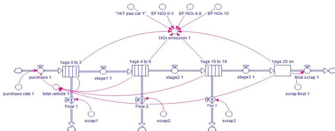
Figure 4.6 The passenger car cohort model with leakage
