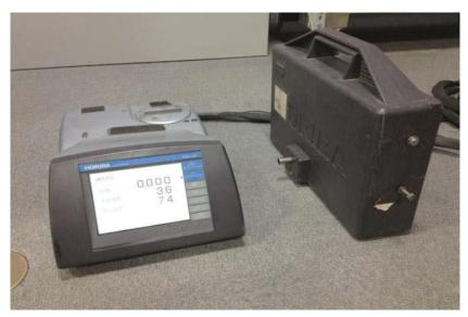
Figure 5.7 MEXA-130S PM analyzer
