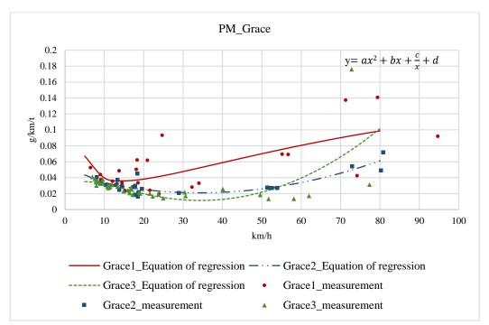
Figure 5.10 EF of PM vehicle with diesel engine
