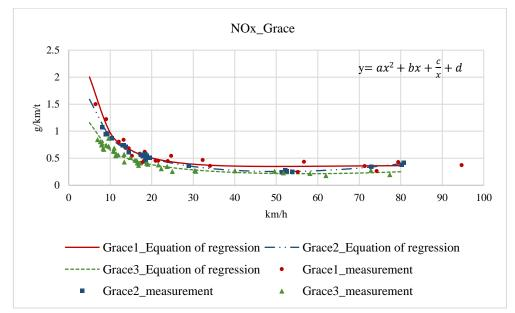
Figure 5.9 EF of  $NO_x$  vehicle with diesel engine
