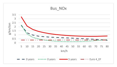
Figure 3.11 Emission factor measurement of bus\_NOx
