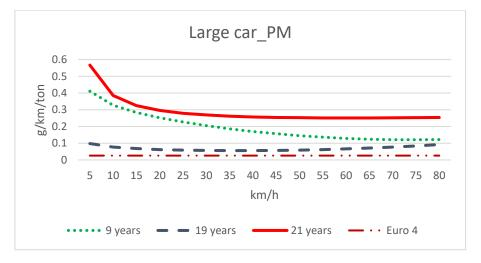
Figure 3.10 Emission factor measurement of large car\_PM
