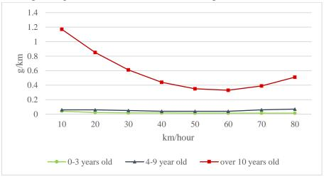
Figure 4.5 Passenger car (gasoline), emission factor of NO<sub>x</sub>
