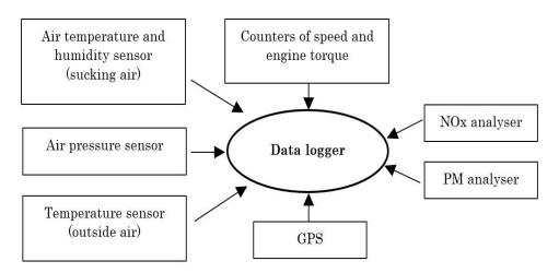
Figure 5.5 On-board emission measurement system scheme
