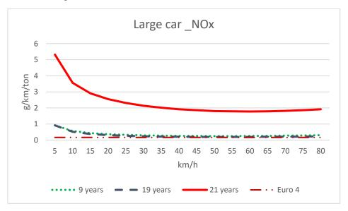
Figure 3.9 Emission factor measurement of large car\_NOx
