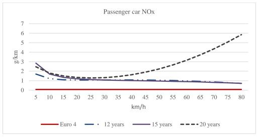
Figure 5.15 EF measurement of passenger car
