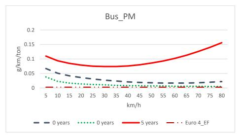
Figure 3.12 Emission factor measurement of bus\_PM
