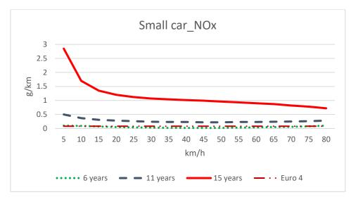
Figure 3.8 Emission factor measurement of small car
