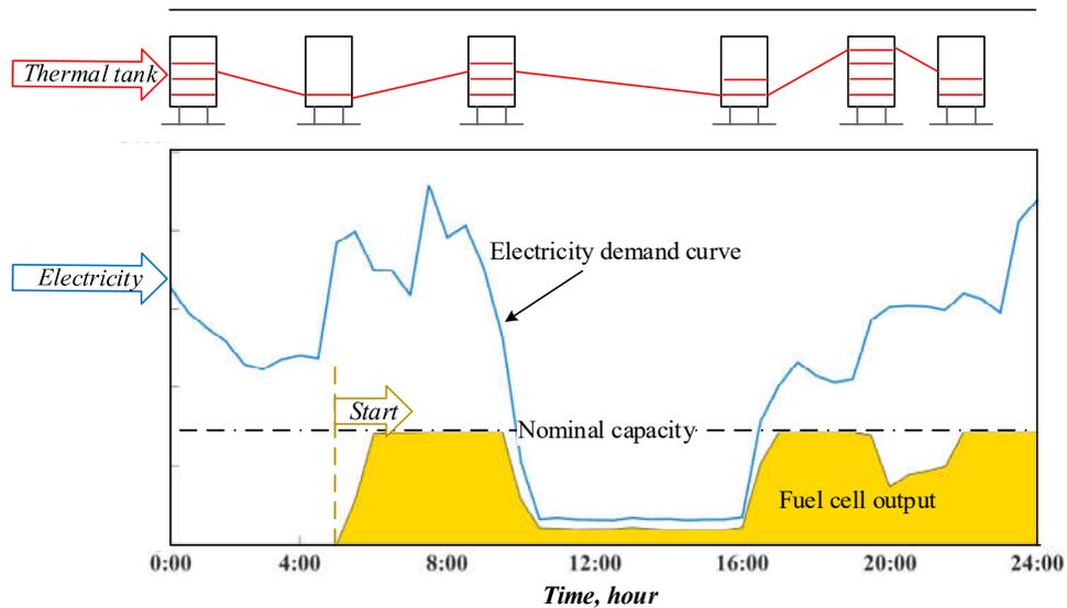
**Fig.5-35. Operational CHP mode of fuel cell in a typical day**
