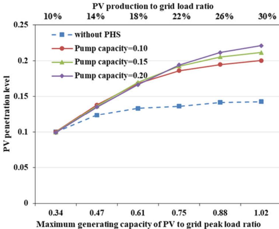
**Fig.4-26. Impacts on effective PV integration of different relative PV capacity with different pumping capacities of dispatch PHS**
