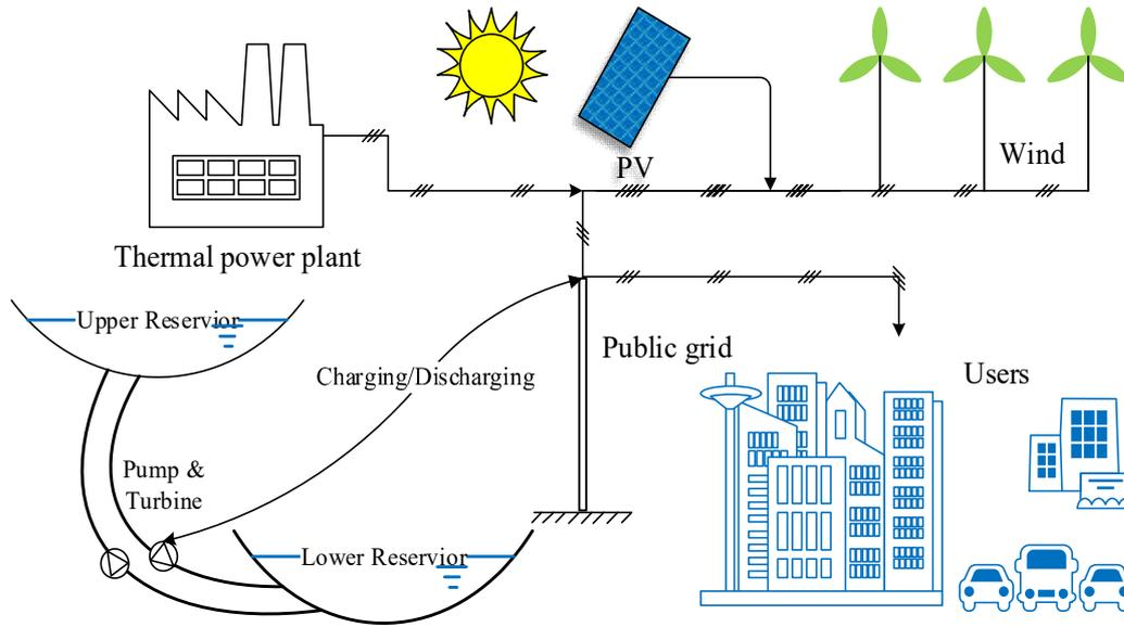
**Fig.2-4. A structure of hybrid power supply system with aid of pumped hydro station**
