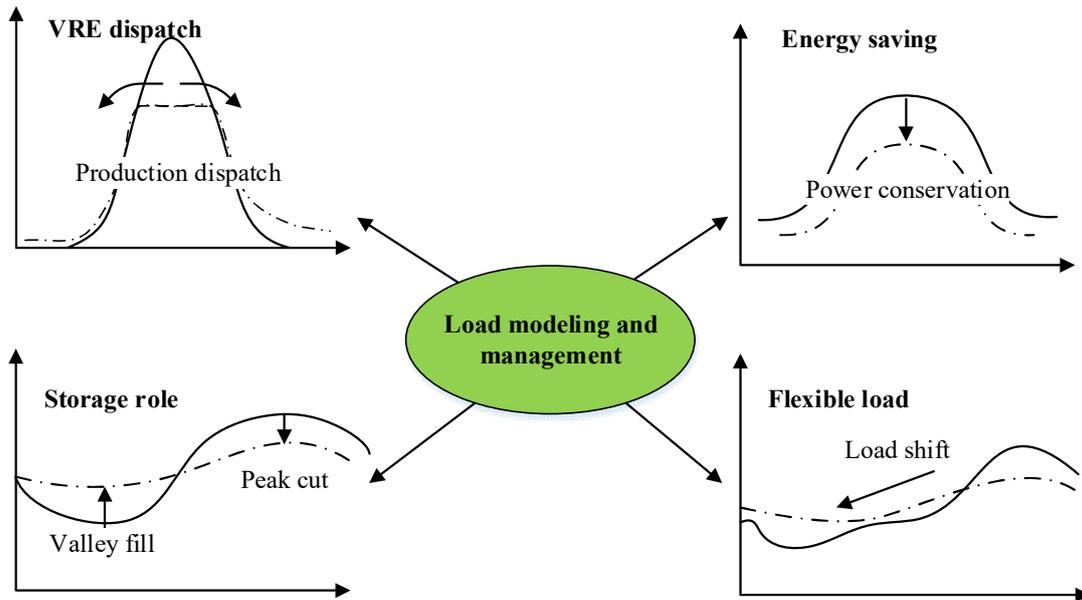
**Fig.1-20. Main activities for load modeling and management in power supply-demand system**
