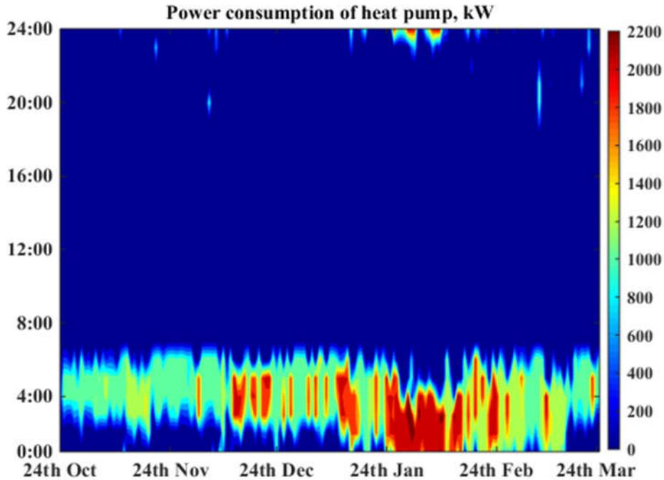
**Fig.5-13. Color scale distribution of power consumption of heat pump sector in a typical residential house**
