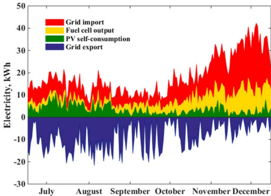
Fig.5-38. The daily power balancing situation for the ZEH with grid-tied hybrid power system
