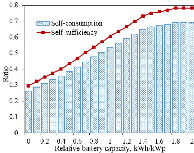
**Fig.5-29. Self-consumption ratio and self-sufficiency degree of residential PV system (5.0 kWh) with different relative battery capacities**
