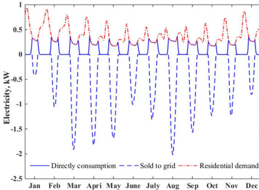
**Fig.5-27. Power flows of the grid-connected residential PV system, 5.0 kW<sub>p</sub> capacity without battery storage**
