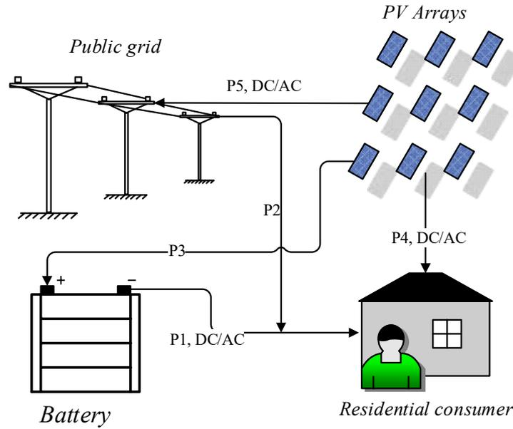
**Fig.5-25. Layout of the grid-connected residential PV-battery system**
