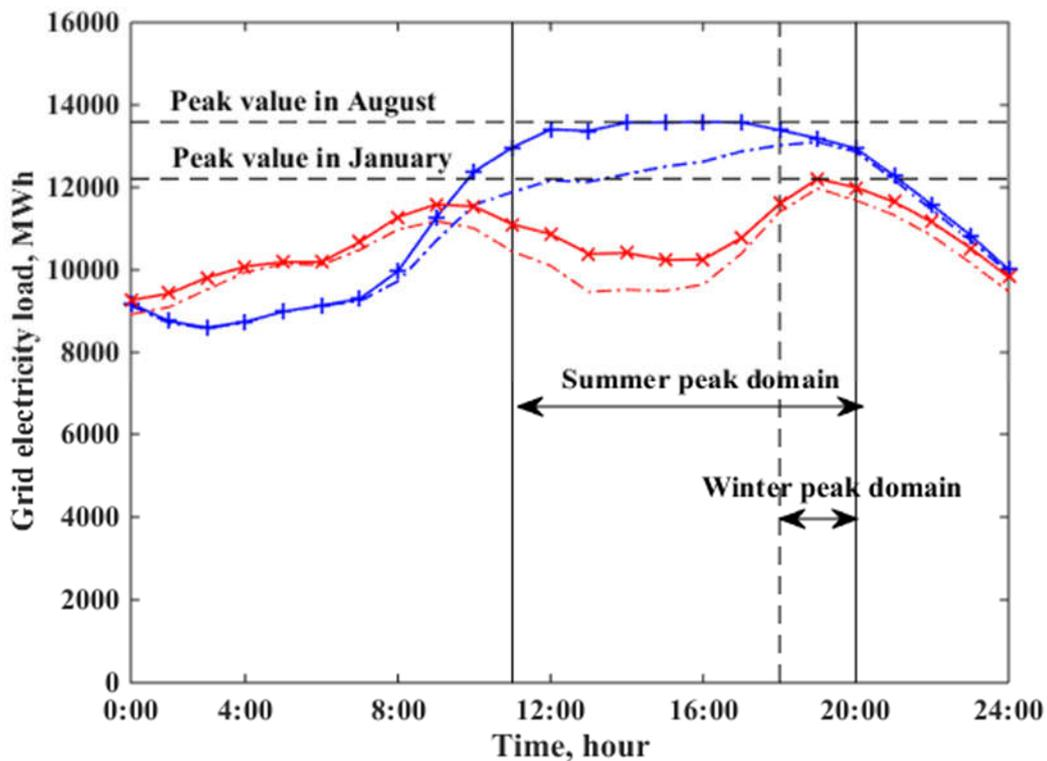
**Fig.6-9. Grid load profiles and peak period domains, and adjusted load profiles with participation of 500 thousand ZEH in Section6.4.**
