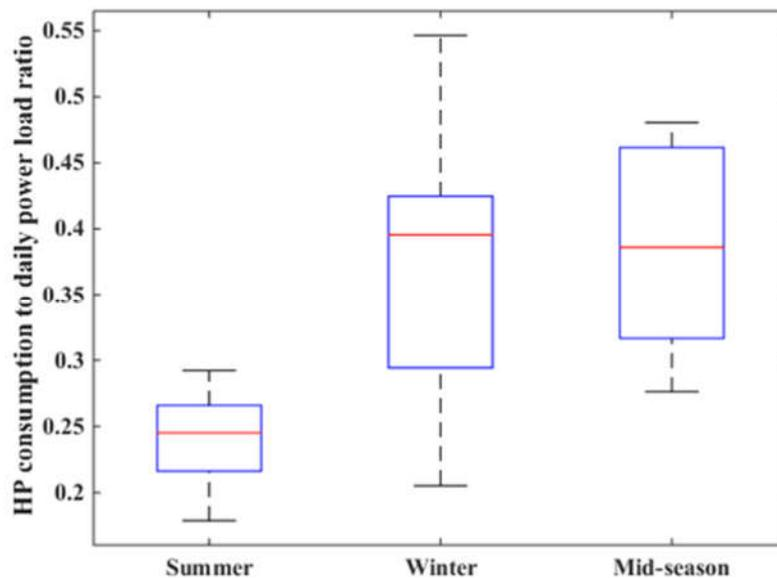
Fig.5-12. Distribution of power consumption of heat pump water heater to daily power load ratio
