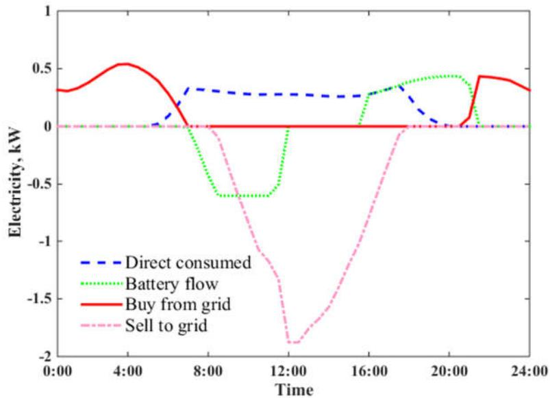
**Fig.5-30. Power dispatch for the grid-connected household PV-battery system in August, PV capacity 5.0 kW<sub>p</sub> and battery size 3.0 kWh.**
