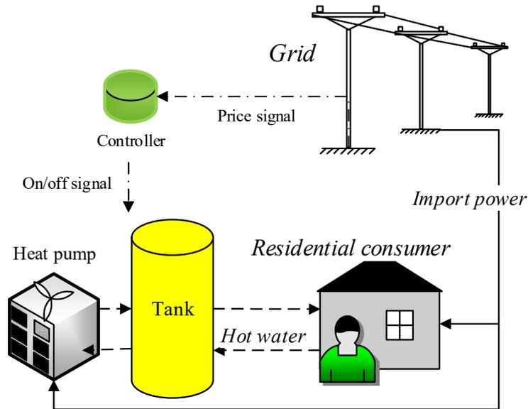
**Fig.5-6. Scheme of residential household with heat pump water heater system**
