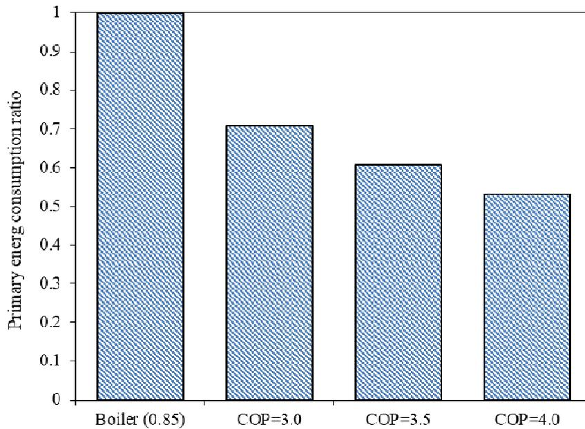
**Fig.5-5. Primary energy consumption ratio of conventional thermal boiler and heat pump**
