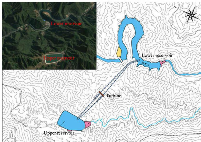
**Fig.2-5. The layout of pump storage station in Omarugawa District, Kyushu**
