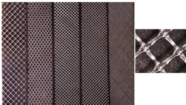
Figure 5-3 Conventional net-type spacers mentioned Lee et al. study [3].
