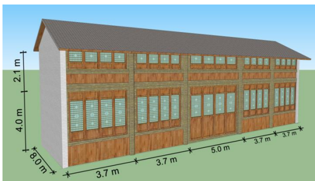
Fig. 3.3 Front facade details and size description of building model in simulation
