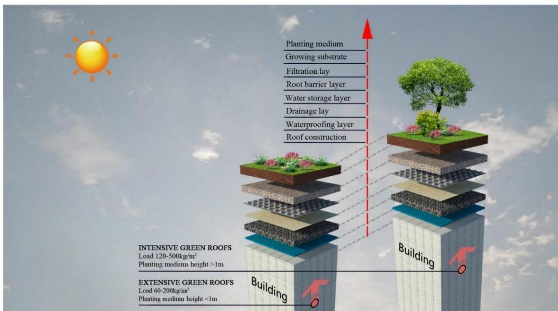
**Figure 1-6** The configuration of intensive green roofs and extensive green roofs
