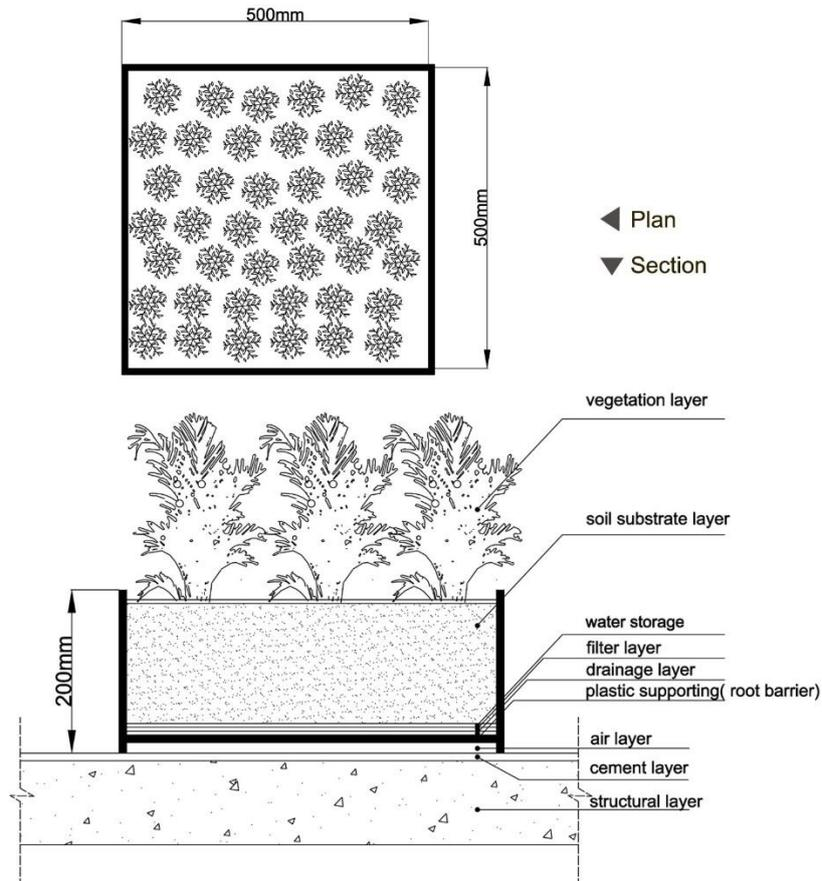
Figure 6-3 The construction of planting beds: plan (top) and cross section (bottom)
