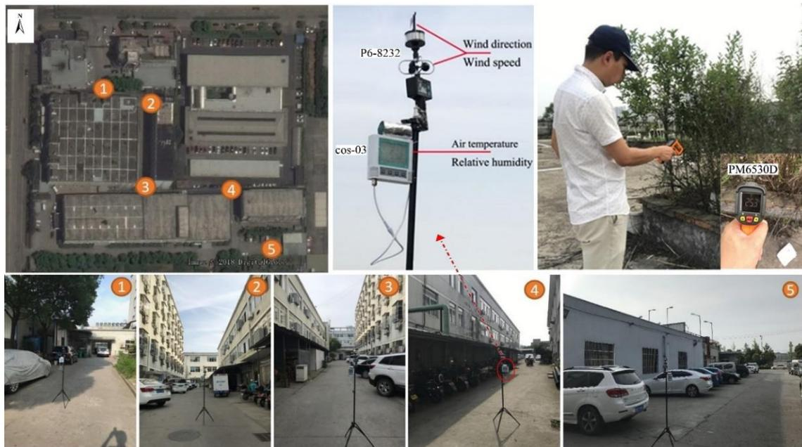
**Figure 4-4** On-site field measurement and the spatial distribution of test points
