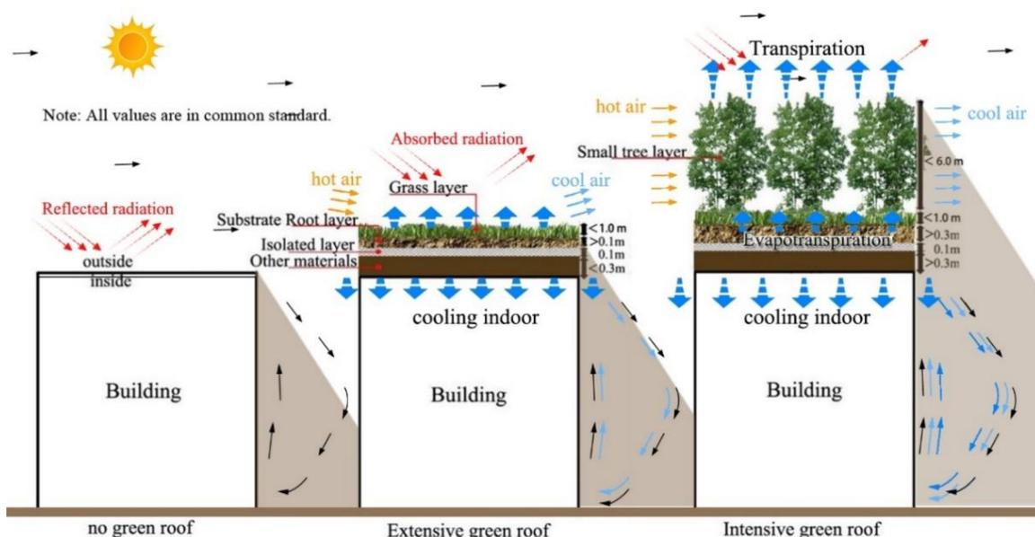
**Figure 1-9** A schematic structure of an extensive green roof and an intensive green roof, and the cooling mechanism in the daytime
