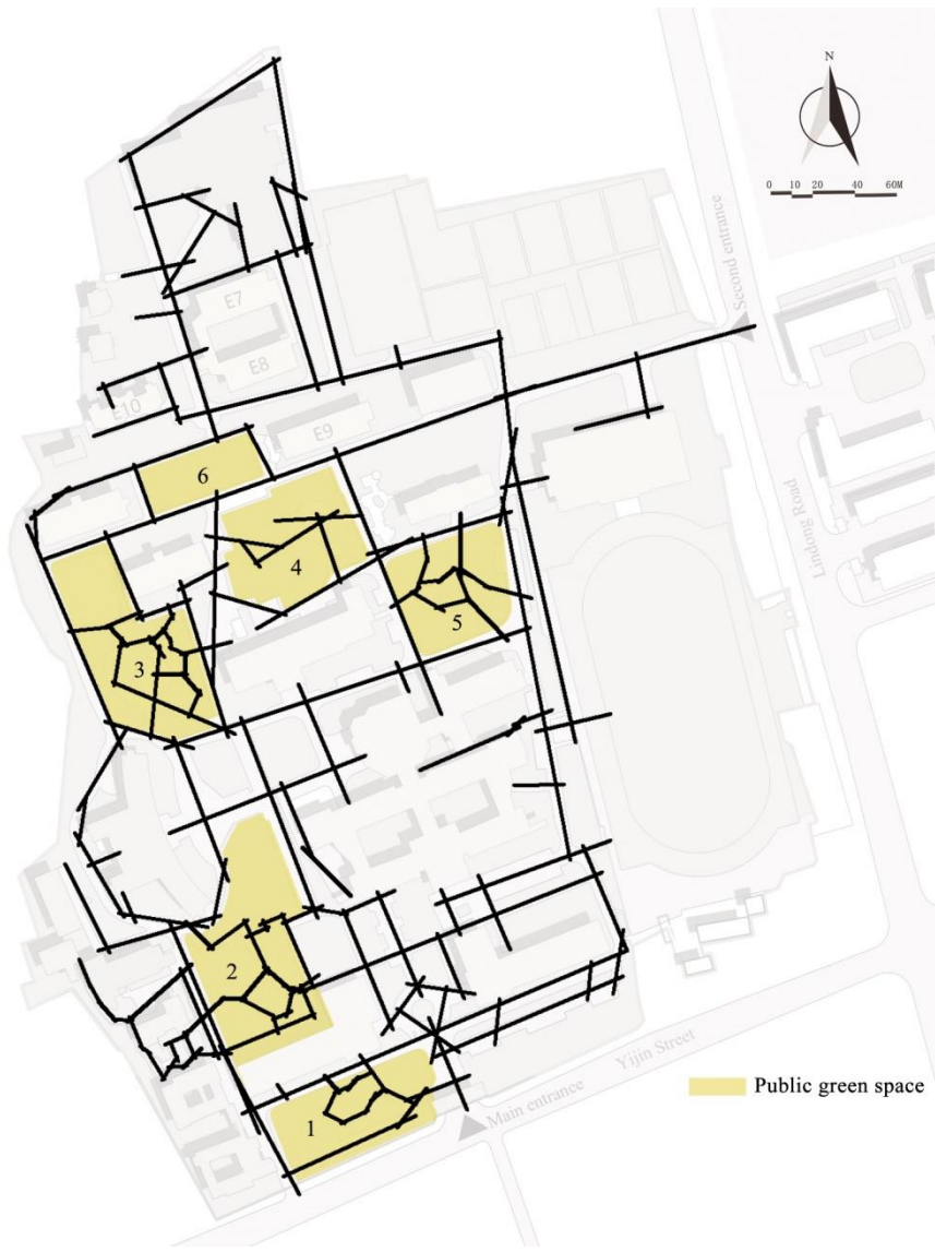
Figure 5.1 Axial line analysis of Yijin Campus based on Space syntax.
