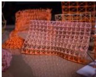
Plate 15 - Experiment 5: Robotic 3D spatial printing
