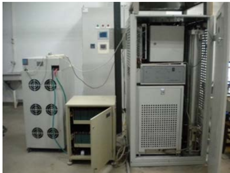
Fig 4-1 Methanol reforming hydrogen production PEMFC experimental platform
