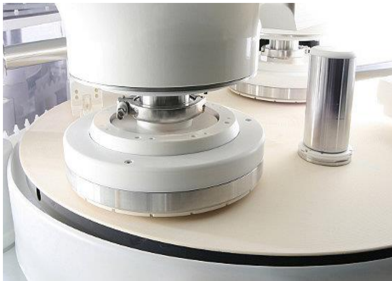
Figure 2.11: A physical picture of the CMP process in VLSI fabrication [41].
