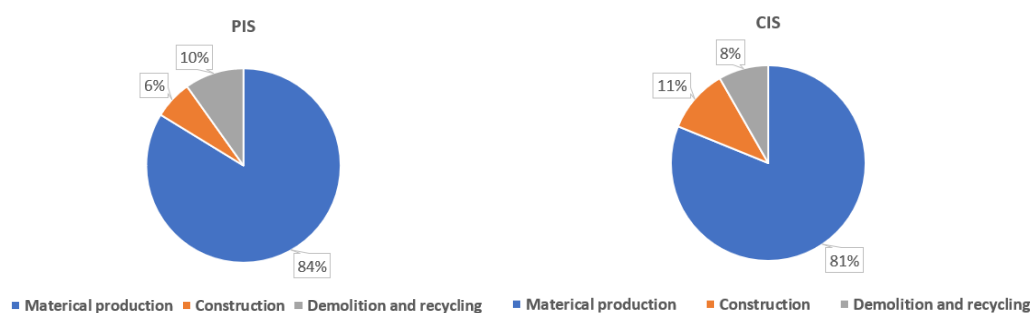
Figure 5.16. Percentage of carbon emissions at various stages of the PIS and CIS.
