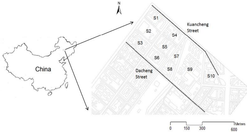
Figure 5.1 Location of target area and planning for drain replacement project (target area was divided into 10 sub-catchments, S1, S2...S10)
