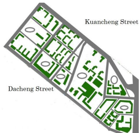
Figure 5.2 Planning for Sponge City (map scale is 1:15,000, green areas are green roofs and grey circles are sand ponds)
