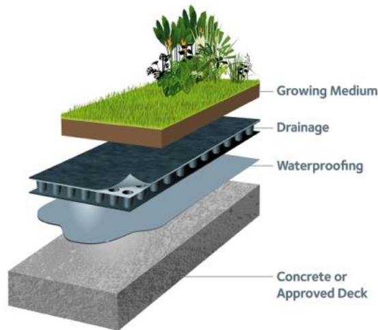
Figure 4.11 Extensive Green Roof technology (Approved desk introduced in this study is plastic tanker, which is lightweight and could be moved easily).
