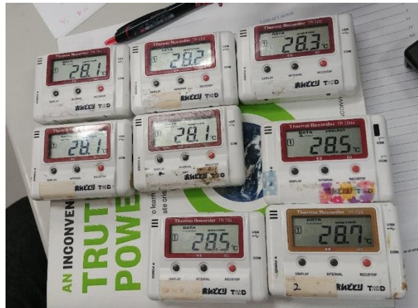
Figure 4. 7. T&D data logger type TR-72U for recording indoor temperature.
