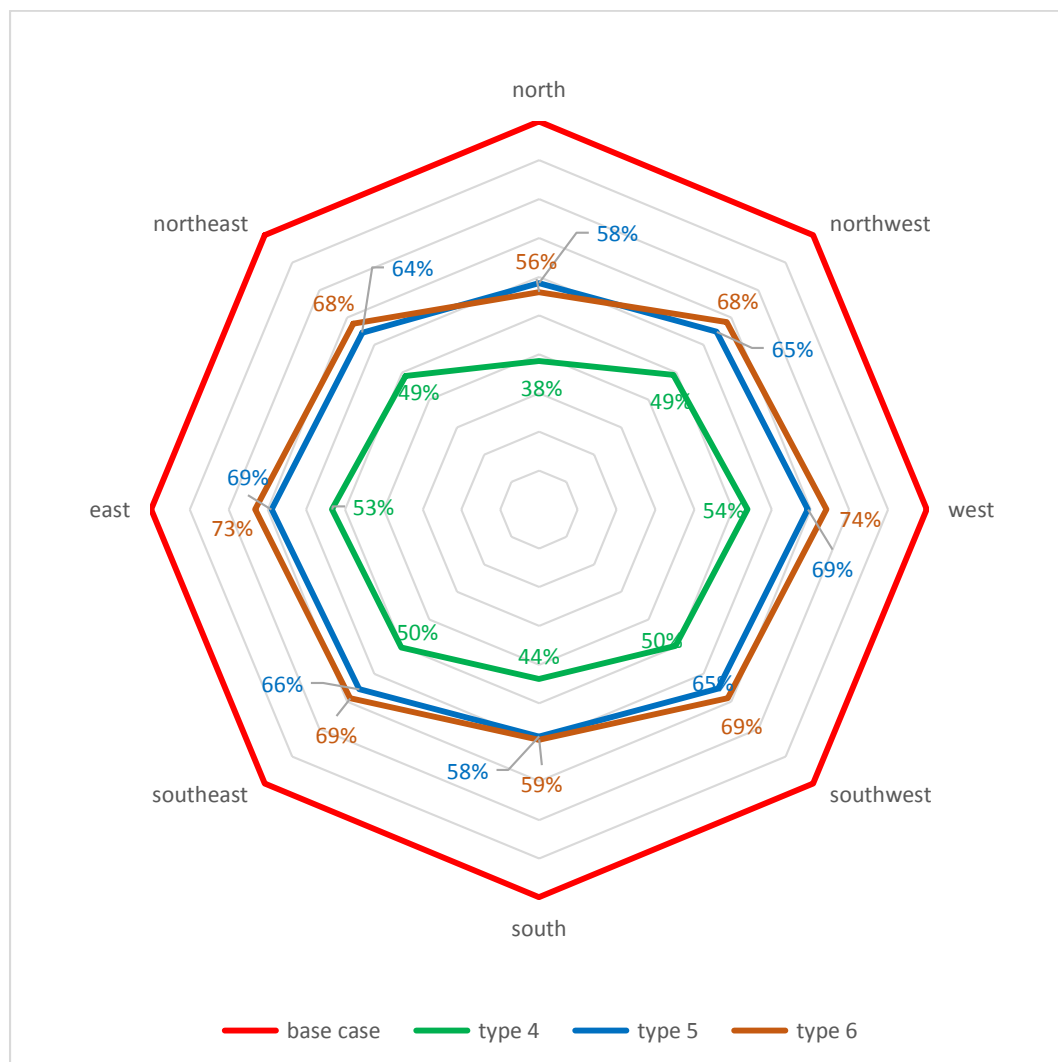
Figure 3. 11. The total solar radiation of the base case in comparison with the type 4, type 5, and type 6 L-shaped mini-louvers.
