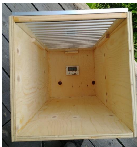
Figure 4. 8. Temperature recorder placement in the middle of the base inside of the box.
