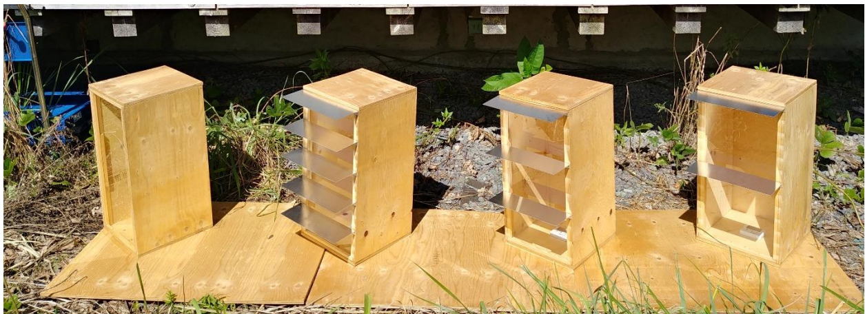
Figure 4. 11. The experiment setting of one base case box without sun shading and three boxes using mini overhangs.
