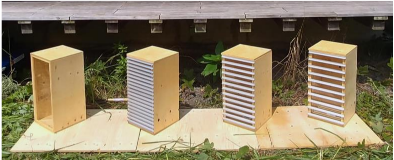
Figure 4. 10. The experiment setting of one base case box without sun shading and three boxes using L-shaped mini louvers.
