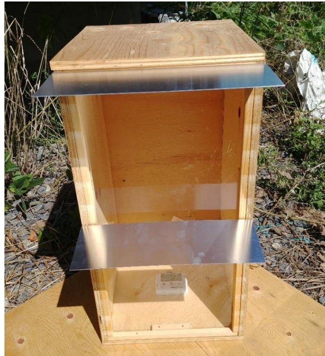
Figure 4. 9. The model D is shown in the picture with thermal recorder inside.
