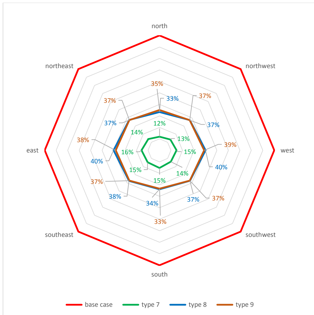
Figure 3. 12. The total solar radiation of the base case in comparison with the type 7, type 8, and type 9 L-shaped mini-louvers.
