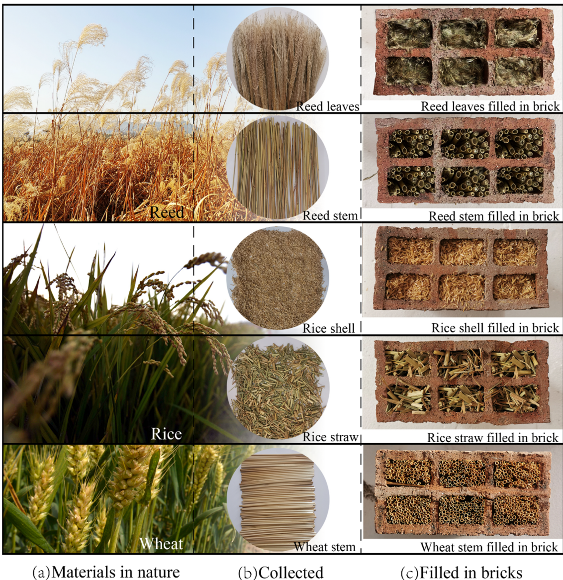
Figure 5.2. Straw and the samples of straw hollow bricks
