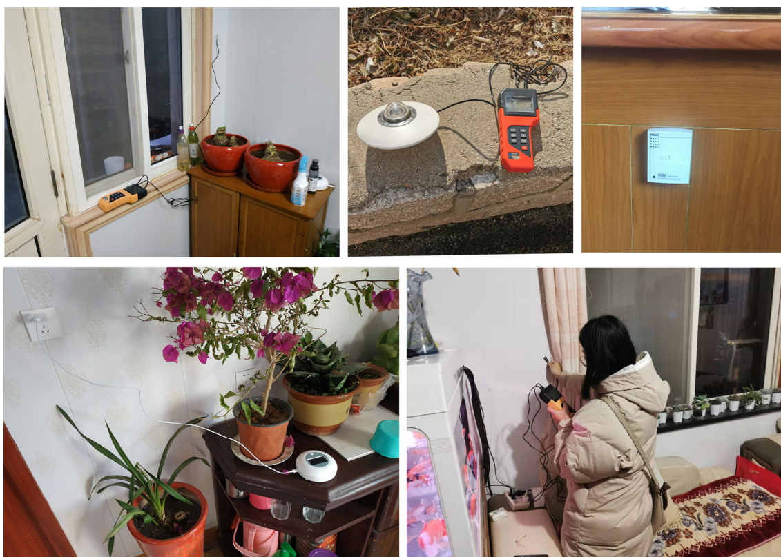
Figure 4.24. Photographs showing examples of field measurement of indoor air quality
