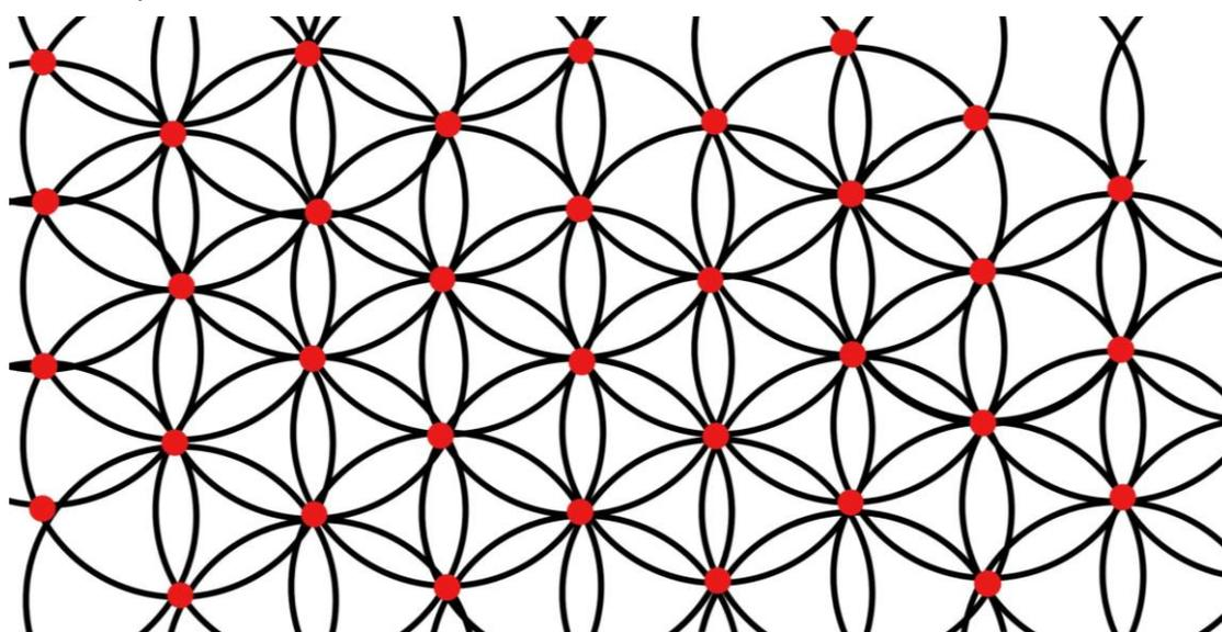
Figure 4-3 A circle into six equal parts with a compass and draw a rose pattern
