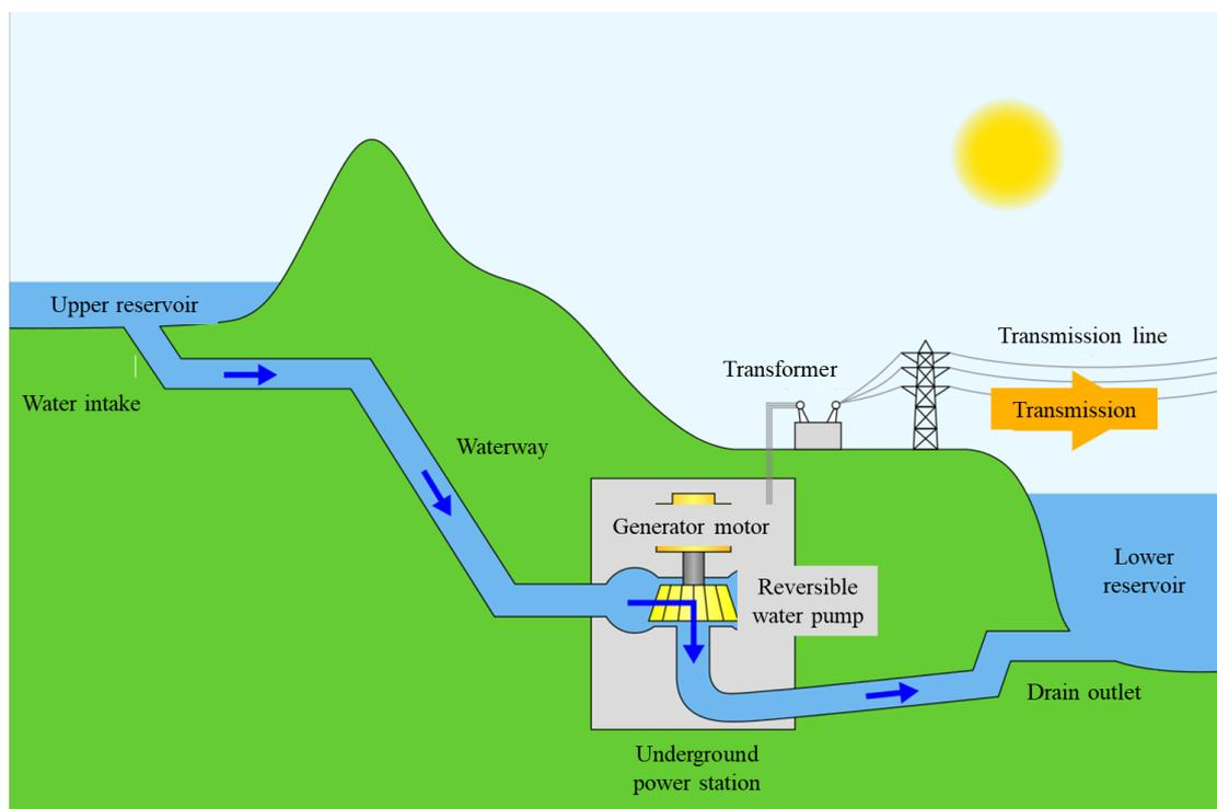
**Fig. 3-8 The configuration of PHS interconnected [13]**
