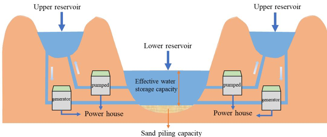
**Fig. 3-11 Basic layout with main parameters of the PHS with dams**
