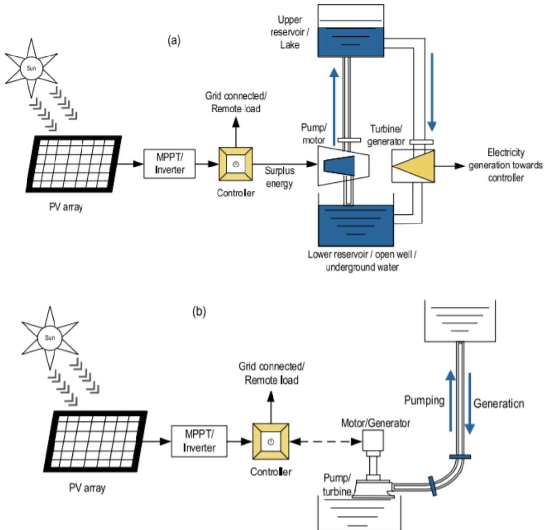
**Fig. 2-8 A hybrid solar-wind system with PHS (a) with two penstocks (b) with single penstock [121]**
