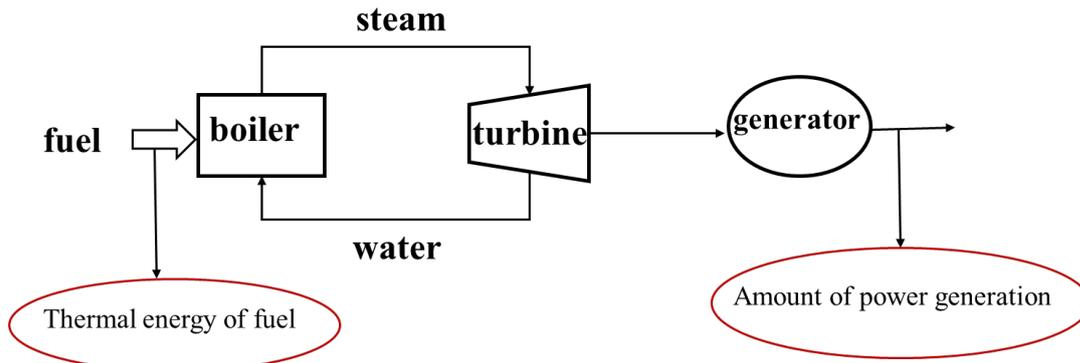
**Fig. 4-23 Flowchart of thermal electricity generation**
