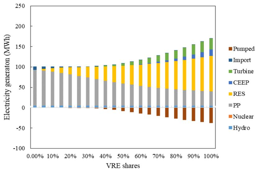
**Fig. 7-27 The configuration of electricity generation under the circumstance of PHS and nuclear power facilities**
