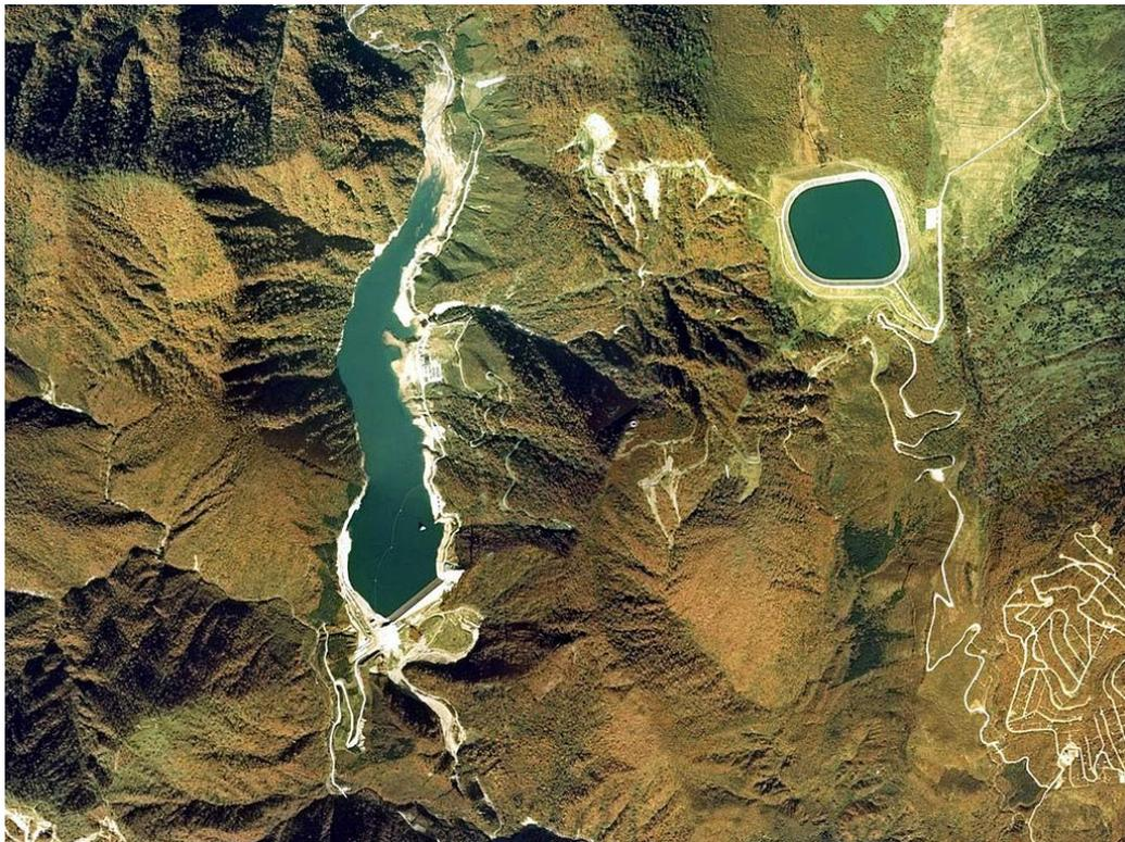
**Fig. 3-9 A pure pumped storage power plant with a dish-shaped artificial lake as an upper pond**
