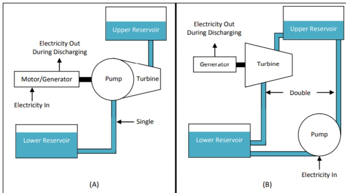
**Fig. 3-17 One PHS facility with (A) a single penstock system and (B) a double penstock system [18]**
