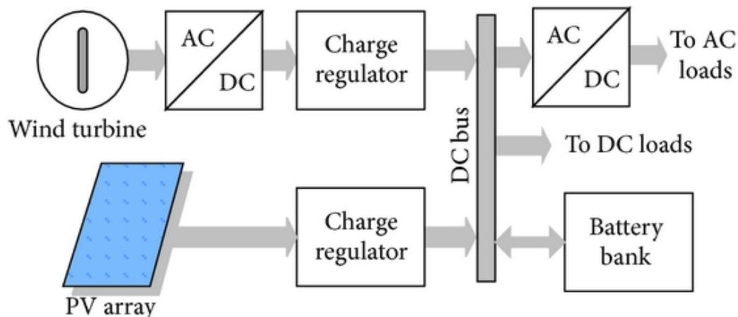
**Fig. 2-7 Grid-connected hybrid system at common current converters [29]**
